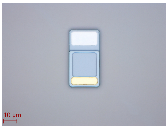
Figure 7.32: Microscope image of the v4 VCSEL with formed mesa and both ohmic contacts.
