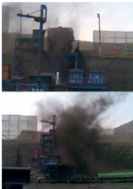
FIGURE 2 Dust float during discharging
