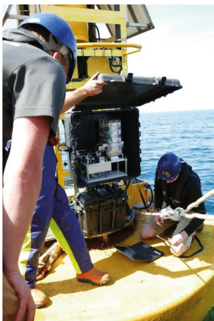
NERC cartridge MAPS design installed at L4 station of the Western Channel Observatory (Credit: NERC).
