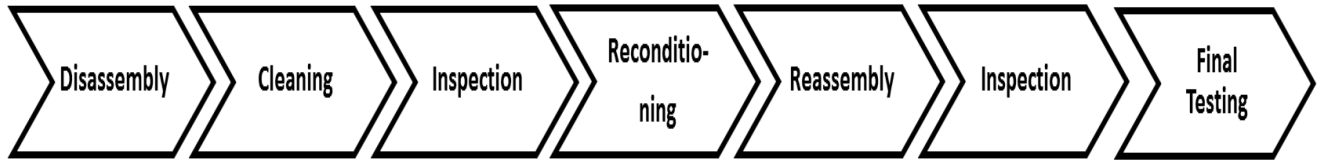
Figure 2: A generic remanufacturing process chart, based on the steps described in Steinhipher [24]
