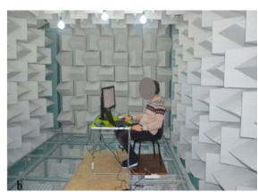
Figure 8. Experimental setup (a) and conduction of the perceptual test (b) inside the anechoic chamber.
