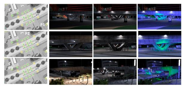
**Figure 3.** The three camera positions and the corresponding images of the three lighting scenarios (from left to right column: Camera position; current situation; functional project and scenographic project).
