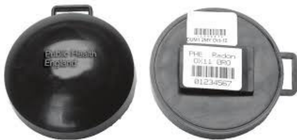
Figure 1. Passive monitors used by PHE to measure indoor radon concentrations.
