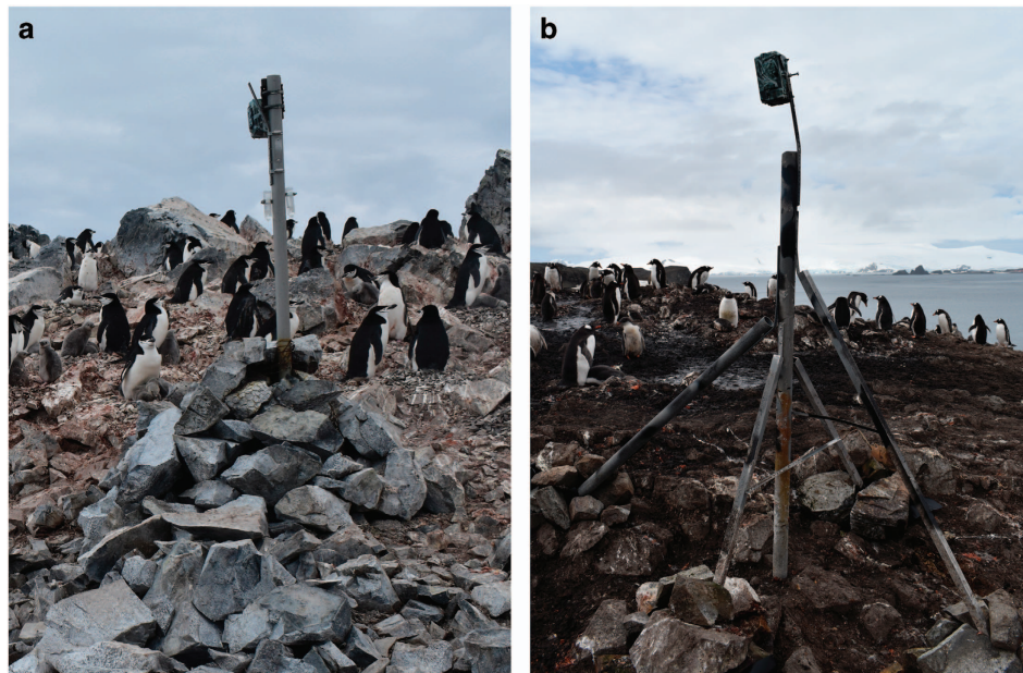
Figure 1. Two examples of remote camera structures. (a) A wire rock basket, covered by further rocks, is used to support the metal scaffold pole (Orne Harbour, Antarctic Peninsula); (b) multiple metal “legs” are fastened to the main structure for support; each “foot” is secured using rocks (Aitcho Islands, South Shetland Islands, Antarctic Peninsula). The design shown in (b) is favoured for future constructions as the “legs” provide increased stability and are longer-lasting than the wire used in (a), which becomes brittle after approximately three years. The cameras shown here are powered by internal batteries. Photo credit: FMJ.
