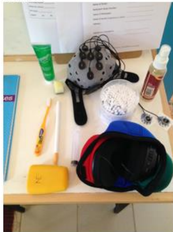
Picture 3. Items to have ready when testing: Signa Gel, prepared inner cap, cotton buds, tape remover, toothbrush, charged Necbox, outer cap with charged headphones NOT IN THE PICTURE: Syringe and fresh tip.
