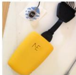
Picture 8. Fibres connected to Necbox, on/off switch in bottom right corner
