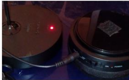
Picture 4. Charging of the headphones. Red light on antennae indicates that headphones are charging. Light turns green when antenna audio jack is connected to laptop and active
