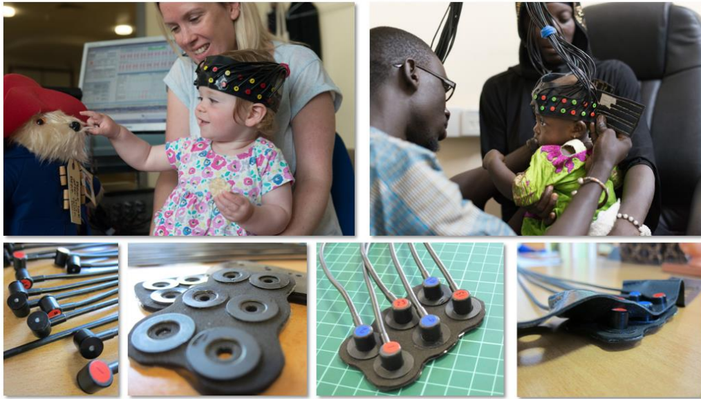
Figure 2.6. Reproduced from Katus et al., (under review) Upper panel; fNIRS headgear worn by infants in the BRIGHT project in the UK and The Gambia. Lower panel; optodes and fibres (far left), sensor arrays with clip-on optode holders (left), source (red) and detector (blue) fibres clipped into array (right) and headband and optode array combined (far right).
