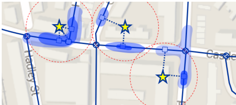
Figure 6.1: Candidate positions for each GPS observation could be sampled from a realistic complex distribution (shaded in blue) around each observation which we could learn from data.
