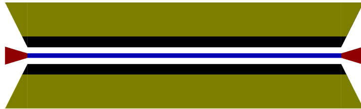
(c) Image showing mask of a single IJJ transmission line. The gold coated contact pads are highlighted in red and the central line is highlighted in blue. The black regions either side of central line are ground contact pads and are connected to ground through gold bonds made to the gold coated region of the ground contact (shown in yellow).
