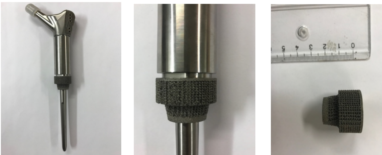
Fig 5.1 A- Proximal femoral implant B- Implant porous shoulder C- Porous Collar
