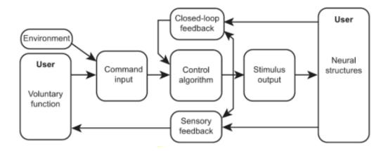
Fig. 2.5 Typical flowchart showing various stages of neuroprosthesis between device (user input) and neural interface to restore motor movements after an SCI. [83]
