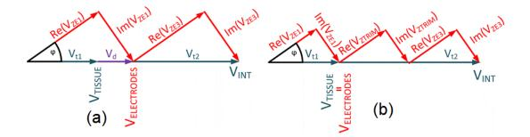
Fig. 3.2. Figure showing phasor representation for bridge of fig. 3.1. (a)  $R_{t1} >> R_{t2}$  but  $Z_{E1}=Z_{E3}$ , the source voltage follows the current through electrodes by phase difference  $\omega_{ZE1} = \omega_{ZE3}$ . (b) Ztrim added to balance the bridge that has the phase with phase difference at that frequency,  $\omega_{ZTRIM}=\omega_{ZE3}$ . Figure updated from [164]
