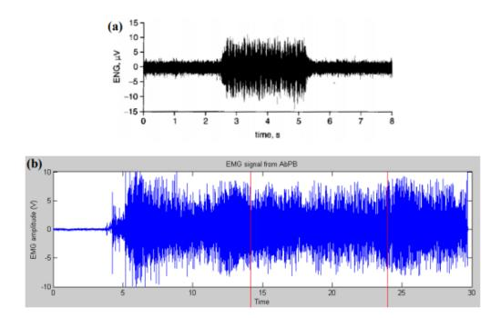
Fig. 2.15 (a) Mechanically ENG spectrum recorded from pig's sacral nerve using tripolar cuff electrode. Trace from Donaldson et al., 2003 (b) EMG spectrum showing amplitude in mV, recorded for about 30s, from the right-hand muscle of a female adult. Graph taken in courtesy from Implanted devices group, UCL.
