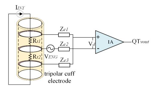
Fig. 2.12 The QT amplifier configuration with tripolar cuff electrode. EMG appears at Rt1, Ze1 and Rt2, Ze3, while ENG forms peak at the middle electrode.
