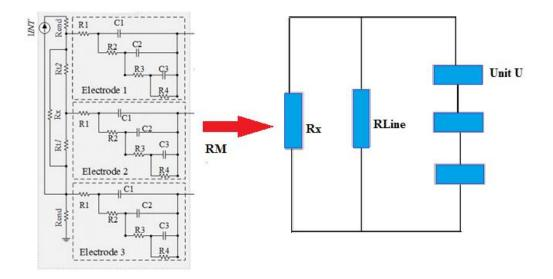
Fig. B. The representative model of book electrode, created using the unit circuit shown in fig. A. where Rline is the combined resistance of Rend, Rt1 and Rt2. Each unit U respresents one ring of tripolar cuff electrode.
