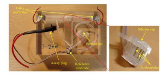
Fig. 3.5 Top figure showing custom setup built to measure the effect of using Ztrim with book electrode for EMG minimisation. Bottom figure shows the picture of actual T-shaped tank used in invitro testings.
