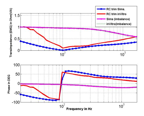
Fig. 3.9. Comparison graph showing EMG minimisation using simple RC as a Ztrim at 100Hz. RC compensation circuit parameters found in simulations (blue line) shows its correlation with invitro results (red line) by minimising EMG (20% imbalance in the book, ~1 V/I interference) by a factor of 10 in invitro in contrast to reduction by a factor of almost 200 in simulations. Results confirm that simple RC when used as a Ztrim is capable of minimising EMG only at the spot frequency.
