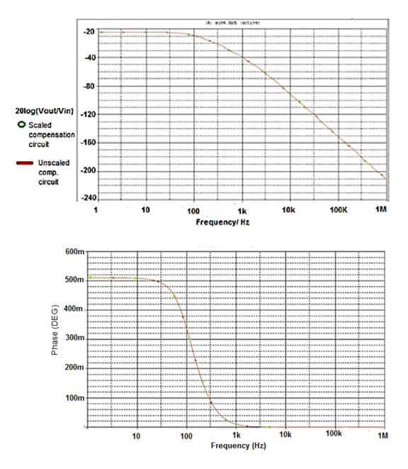
Fig. 3.16 Graphs showing magnitude and phase comparison of the original unscaled 3 stage RC compensation circuit with its scaled version, when resistors were scaled up by the same value when capacitors were scaled down.
