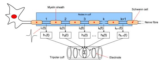
Fig. 2.16 Illustration of SFAP recorded using cuff electrode, due to addition of current sources at each node of Ranvier, delayed by the time td with respect to node k. [figure taken from (Andreasen 1997)].
