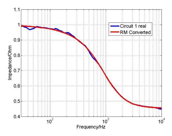
Fig. E. Comparison between RM converted of circuit 1 to the real experimental values of circuit 1
