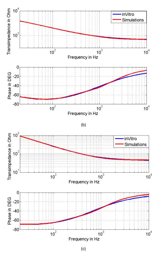
Fig 3.7 (b) Electrode impedance modelling of electrode disc 2 (Ze2) and (c) electrode disc 3 (Ze3) of the book electrode, showing good correlation of proposed 3 stage RC ladder network CPE with the experimental results.
