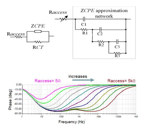
Fig. 3.2. Top figure showing model used for CPE of recording electrode. Bottom phase graph shows, how forcing Ztrim to behave like CPE is achieved using 3 stage RC network by varying active electrolyte bulk resistance, Raccess from 5 $\Omega$  to 5k $\Omega$ .Brown line represent phase output using 5k $\Omega$  and pink line shows for 5 $\Omega$ . Forcing Ztrim to behave like CPE is likely to remove interference irrespective of the frequency.
