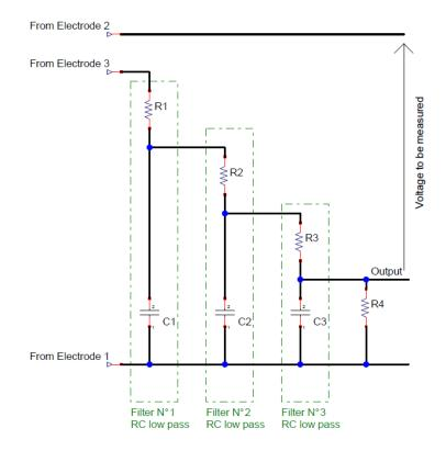
Fig. 3.15 The 3-stage RC compensation circuit that can also be seen as 3 low pass RC filters attached to another.
