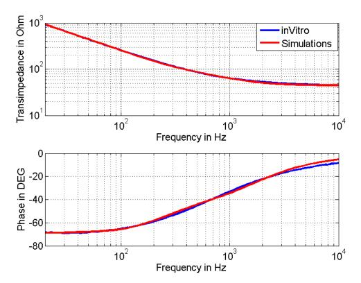
Fig 3.7 (a) Electrode impedance modelling of electrode disc 1 (Ze1) of book electrode, showing good correlation of proposed 3 stage RC ladder network CPE with experimental results.
