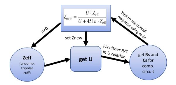
Fig H Block diagram showing the steps that can be taken to calculate the circuit parameters of the compensation circuit required in bringing the output of the tripolar cuff closer to null for EMG minimisation
