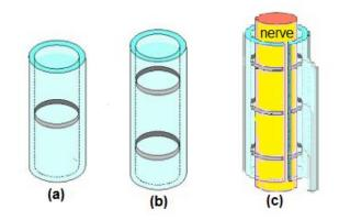
Fig. 2.10 Types of cuff electrodes. (a) monopolar cuff electrode with one ring electrode (b) bipolar cuff electrode with two electrode rings (c) tripolar cuff electrode encapsulating a nerve with three ring electrodes. Figure revised from Pachnis PhD. dissertation, 2010
