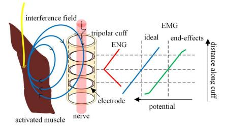
Fig. 2.11 ENG and EMG potential under ideal and real conditions. Muscle activity producing differential-mode interference causing voltage drop in tissue resistance. End-effects exploit cuff linearizing property making EMG unequal between the electrodes and does not result in its complete removal. [114]
