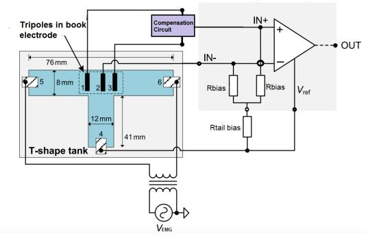
On chip ENG amplifier to be used in implant
