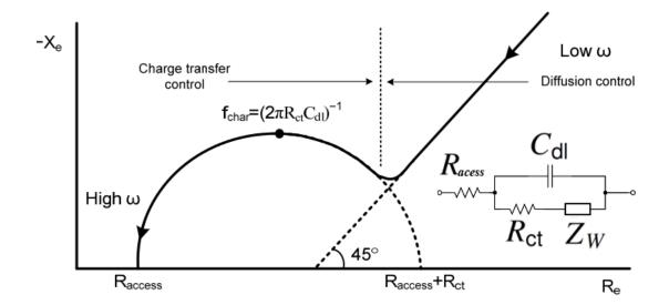
Fig. 2.19 Randles equivalent circuit model on the right. Raccess is active electrolyte resistance, Rct charge transfer resistance, Zw Warburg element. Nyquist plot using Randles model, showing impedance characteristics at high and low frequencies. Bulk resistance is dominating at high frequencies, and ions diffusion process at lower frequencies due to Cdl dominance. Nyquist plot reproduced from [143]
