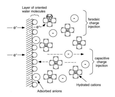
Fig. 2.17 Faradic and non-Faradic charge transfer at electrode electrolyte interface. [136]
