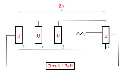
Fig. F connecting 'n' units in parallel to RM of Circuit 1 to create limiting relation for new overall impedance, Zn. See equation 4.
