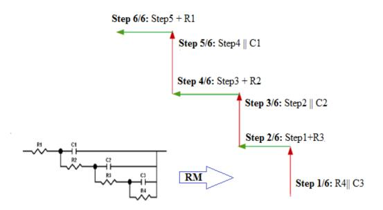
Fig. A Approach considered to build a representative model (RM) of circuit 1(book electrode) using its electrode impedance model
