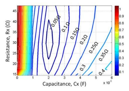
Fig. 3.14. Sensitivity analysis, to check robustness of Rx and Cx parameters in 3stage RC compensation circuit in achieving a certain EMG minimum. Transimpedance values obtained for each combination are shown on the contour lines. The suitable range for Cx is beyond 1uF and for resistors below  $18\Omega$ , after which differences from the minimum rise much more gradually.
