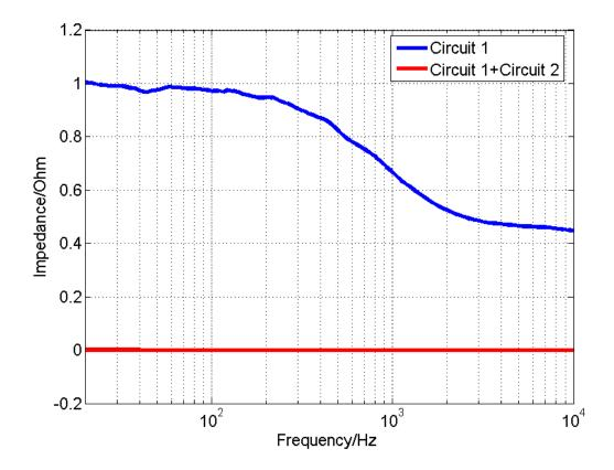
Fig. G Output results of  $Z_{new}$  when circuit 2, compensation circuit is attached to circuit 1. It shows that when only one unit is attached it forces the output close to null. Also, output response of circuit 1 and 2 is not a flat line but ranging between  $1.6m\Omega$  to  $1m \Omega$ , with becoming constant at higher frequencies
