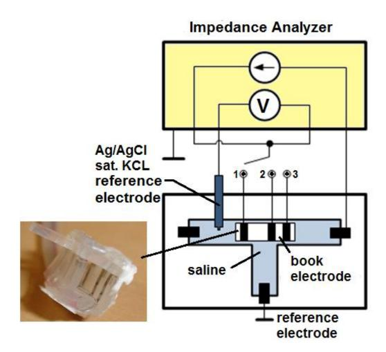
Fig. 3.4 Test apparatus used to measure impedance of electrodes in the book arranged in tripolar configuration (middle electrode offset). Ag/AgCl sat. KCl was used as a reference electrode and transimpedance was recorded for each electrode using impedance analyser. Picture on the left shows the real book electrode used in the tank.
