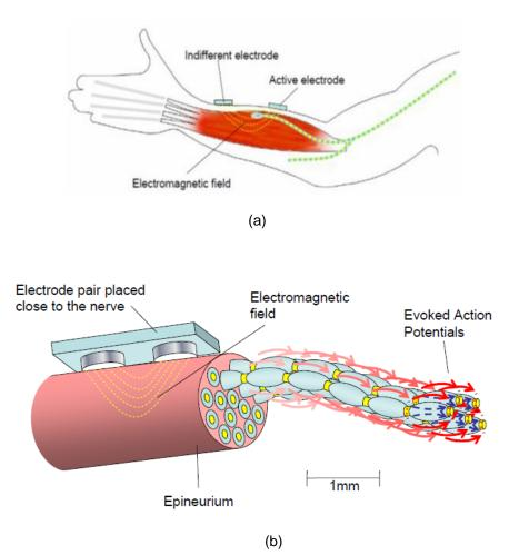
Fig. 2.7. Types of electrodes that are used in FES systems to record neural signal. (a) Surface electrodes, (b) Implanted electrodes [103]
