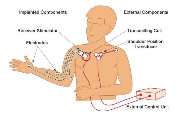
Fig. 2.6. shows FES system in use to restore hand grasping and elbow movement. Transducer sends a signal to control unit on shoulder movement, which sends pulses to the effected nerves using implanted electrodes to produce muscle contractions for hand and elbow movement. [88]
