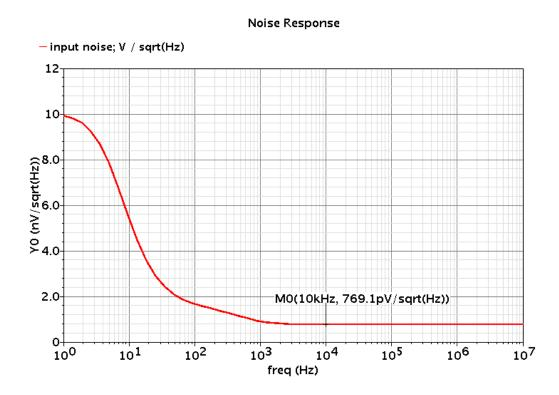
Fig 3.17 Noise response of a 3- stage compensation circuit observed over a longer frequency range, it is evident that noise contribution is more at lower frequencies and almost negligible at higher frequencies.
