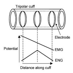
Fig. 2.9. ENG and EMG potentials shown inside the cuff electrode for neural signal recording. [49]
