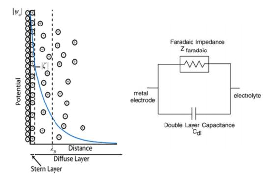
Fig. 2.18 Left figure showing the double layer model by Stern and the right figure shows the equivalent circuit model due to transfer of electrons at equilibrium (Stern layer). [136]
