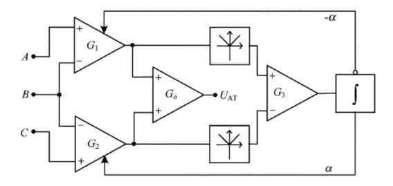
Fig. 2.14 Schematic of the Adaptive-Tripole for EMG minimisation and ENG recording. [112]
