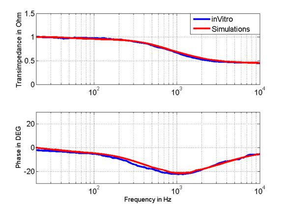
Fig. 3.8. Figure showing the transimpedance spectrum (EMG interference) of imbalanced tripolar book electrode. Simulating book electrode using electrode impedance model shows a close correlation of magnitude and phase with the invitro results, confirming that this book electrode model can now be used in simulation to find Ztrim compensation circuit parameters for EMG minimisation.
