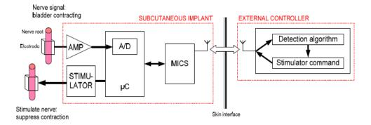
Fig. 1.2a. Block diagram showing the signal pathway between an implant and external controller for stimulating nerve and recording its signal in conditional neural modulator, reproduced from [51]
