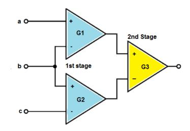
Fig. 2.13. The TT amplifier configuration, a, b and c points are linked to the electrodes in the cuff, EMG is removed but at the expense of more current consumption.
