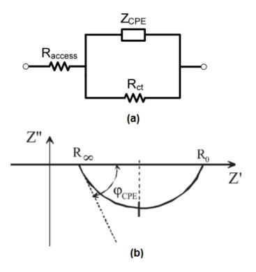
Fig. 2.20 (a) Cole model in which Cdl is equated to  $Z_{CPE}$ . (b) Impedance loci of Cole model,  $R^{\infty}$  showing resistance at high frequencies and  $R_0$  showing resistance at low frequencies. Dotted line shows  $Z_{CPE}$  and  $\phi_{CPE}$  is an angle of CPE. Loci model graph reproduced from [146].
