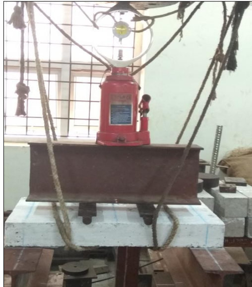
Fig. 3. Slab panel subjected to flexural strength test.
