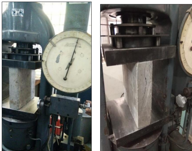
Fig. 6. Wall panel under compression test.
