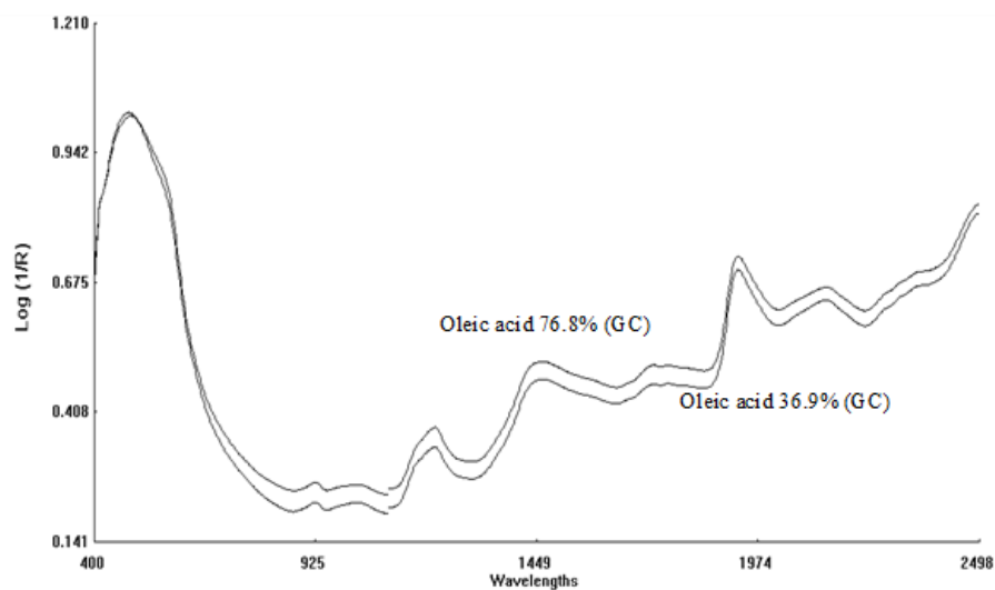
Figure 2. The raw absorption spectra of peanut kernels representing two extreme oleic acid values
