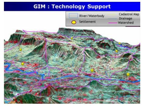
(GIM) technology support has also been initiated and involves the village map geo-referencing through Indian Satellite Images. This involves collection of village map, scanning of map, geo-referencing of scanned map to satellite data and digitization of geo-referenced village map. The figure above illustrates GIM technology.
