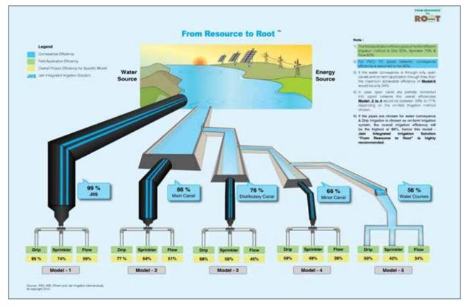
to the field and application is through only drip Irrigation, the overall efficiency of this model is 89%. There is a scope for improving overall efficiency of the project from existing 34 % to 89%. The overall efficiency will depend up on the stage at which we are bringing the technological intervention.
