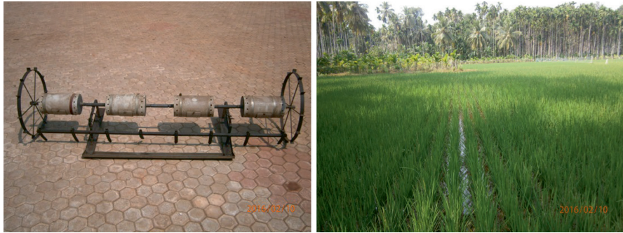
Fig. 8.6 (a) The drum seeder and (b) the crop of wet-seeded rice ( left ) sown by using the drum seeder (Photos by A.N. Rao)
