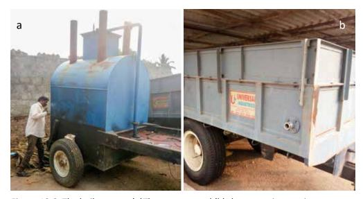
Figure 10.6. The boiler parts: (a)The steamer and (b) the turmeric container.
