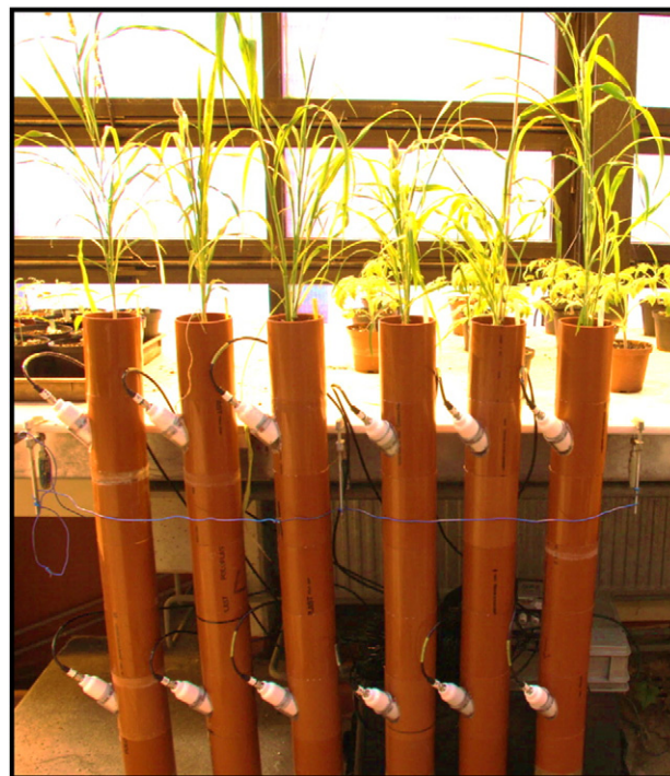
Fig. 1. Application of drought stress to Pennisetum glaucum . Plants are grown under controlled glasshouse conditions in high temperature tubes (HT pipe made of polypropylene, commonly known as PP pipes). Water content is monitored with sensors in the upper and bottom part of the tube.
