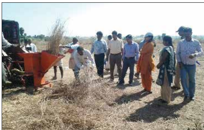
Figure 5. Shredder machine for aerobic composting demonstrated in Idapanur, Raichur District.
