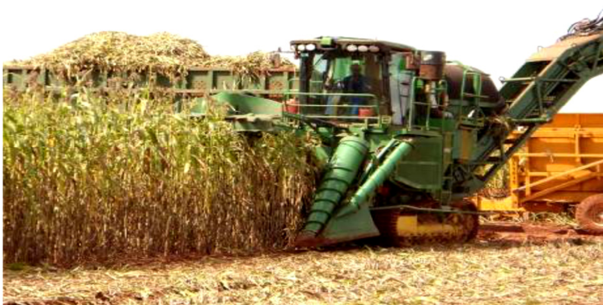
Figure 10: Harvester adjusted for harvesting sweet sorghum (© EMBRAPA)
