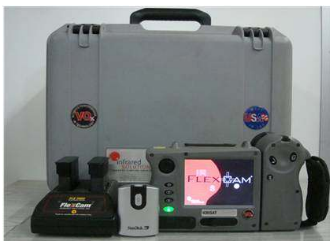
Plate 5: Infrared camera, IR FLEXCAM, used for measuring the crop canopy temperature
