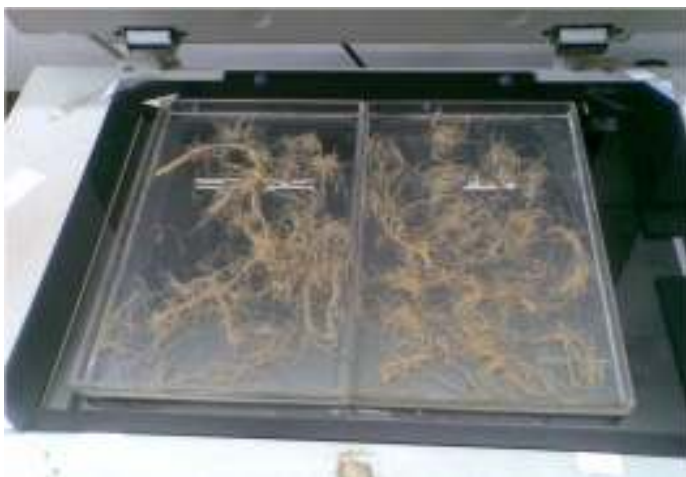
Plate 3: Scanned image of chickpea roots saved as .tif files used for image analysis. The root sample used here is harvested from cylinder culture
