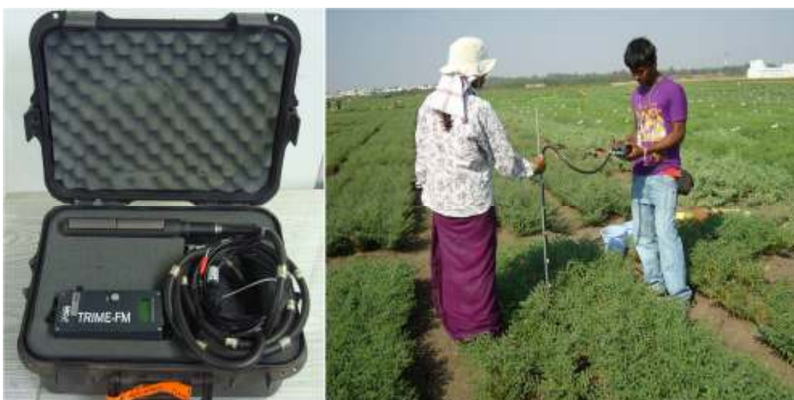
Plate 4: Soil moisture measurement using TRIME-FM TDR (Time-Domain Reflectometry) meter under field condition
