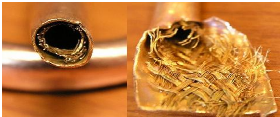
Figure 1.4: Screen Mesh wick ( http://www.frostytech.com )
