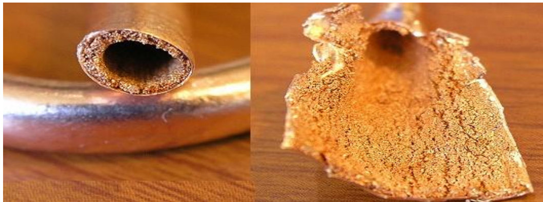
Figure 1.2: Metal sintered Powder wick ( http://www.frostytech.com )
