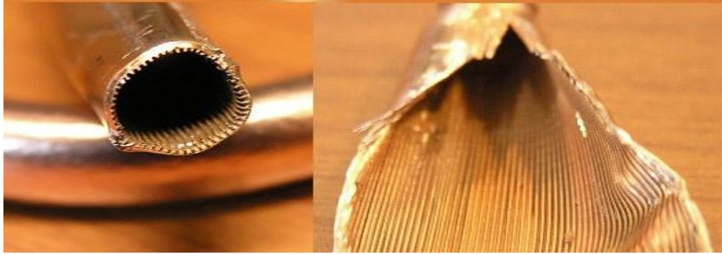
Figure 1.3: Grooved wick ( http://www.frostytech.com )
