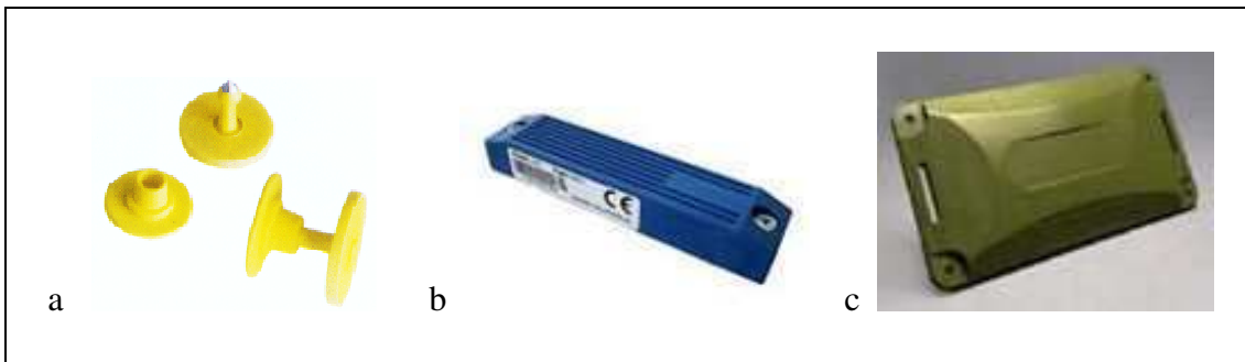
Figure 2.1: samples of active and passive RFID tags ( GAO RFID ) (a): 125 kHz Low Frequency (LF) Animal Tracking Ear RFID Passive Tag ( GAO RFID ) (b): Active RFID UHF –beacon Tag ( GAO RFID ) appropriate for tracking mobile assets (c): A passive UHF (860 to 960 MHz) RFID Tag ( GAO RFID )
