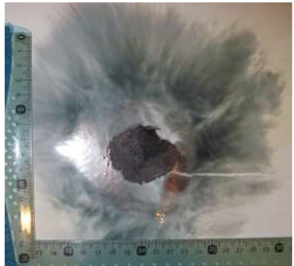
Fig. 4. Typical observable damage after D waveform LS test on a CFRP target.
