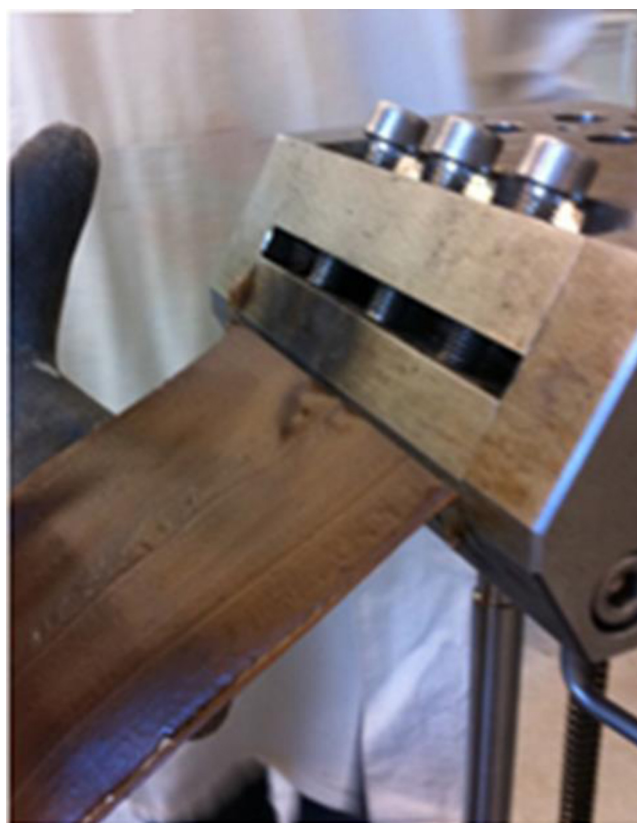
Fig. 1. Sheet production from plasticized wheat bran extract via extrusion. Width of the die is 100 mm and slit thickness 250 \mu m.
