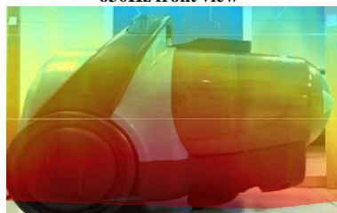
Figure 9. Contour map of sound pressure-velocity (PU) at 630Hz right side view
