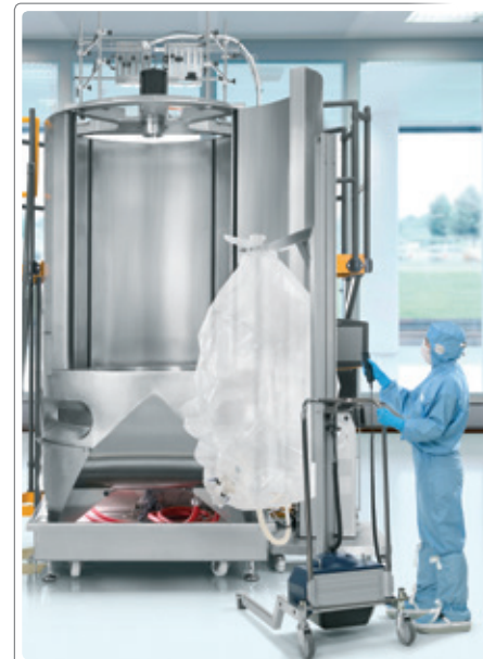
Lifting device for easy installation of 2,000 L bags
