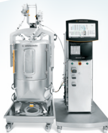
BIOSTAT STR ® 200 50 – 200 L working volume
