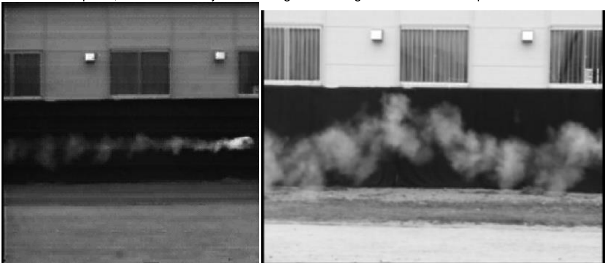
Figure 3: Vortex Pathway for a non-rotating ball viewed from a wide angle (Asai et. al 2007)
