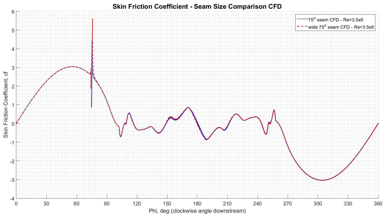
Figure 17: Skin Friction Coefficient Comparison - Single Seam h/b = 2 vs. h/b = 0.17 . (Skin Friction Coefficient was normalized using the following: cf = \frac{\tau_0}{\rho U_\infty} * \sqrt{Re} )
