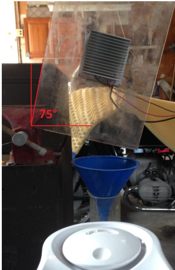
Figure 36. Tilted heatsink experimental setup with 75° tilt.
