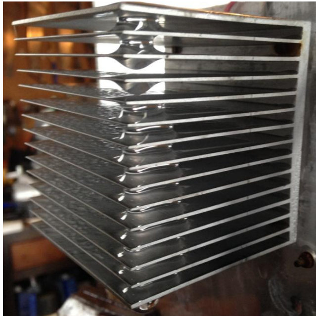
Figure 53. Tilted heatsink timeline condensate bridging at the 1 hour mark.
