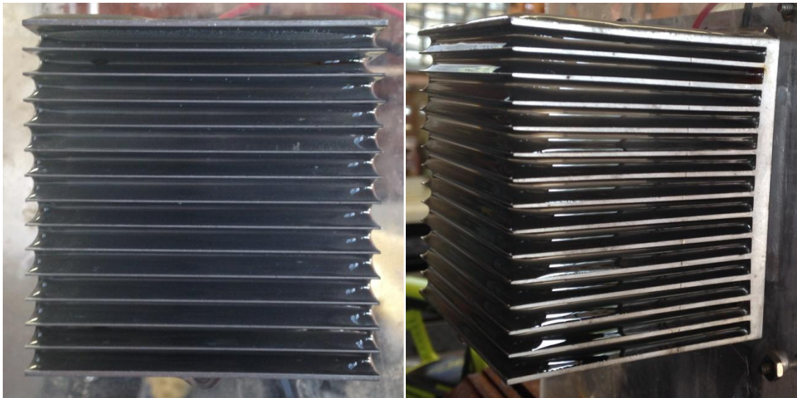
Figure 41. Tilted heatsink split flow condensate bridging at 90°.
