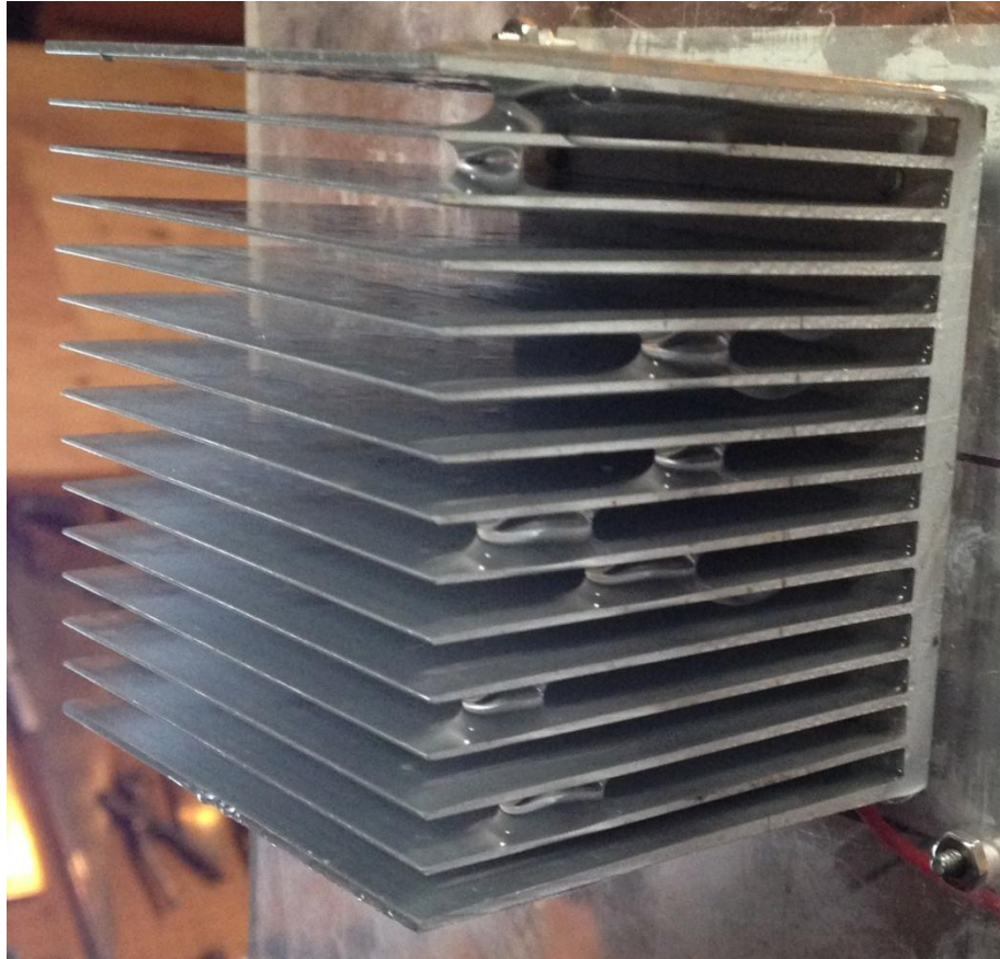
Figure 38. Tilted heatsink split flow condensate bridging at 45°.
