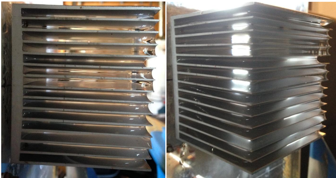
Figure 47. Tilted heatsink through flow condensate bridging at 90° (24 Hr).
