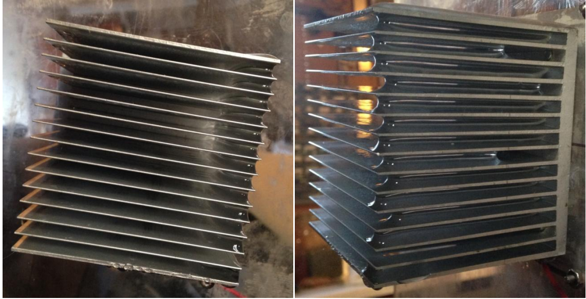
Figure 40. Tilted heatsink split flow condensate bridging at 75°.
