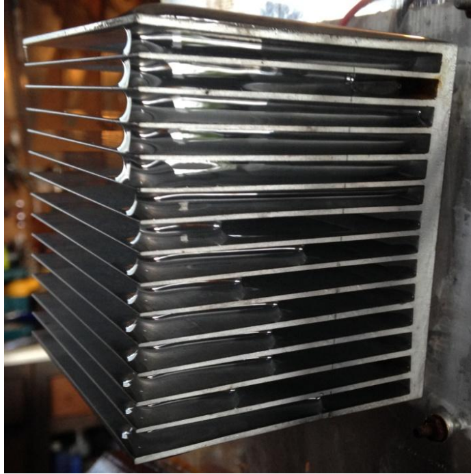
Figure 58. Tilted heatsink timeline condensate bridging at the 6 hour mark.
