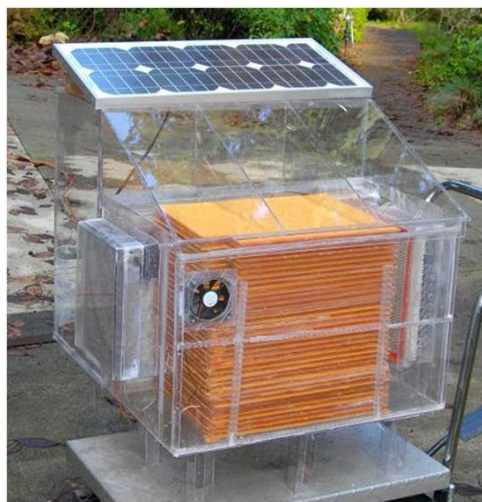
Figure 8. The A2WH active moisture harvester. (11)
