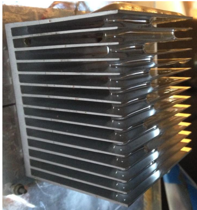
Figure 45. Tilted heatsink through flow condensate bridging at 75°.
