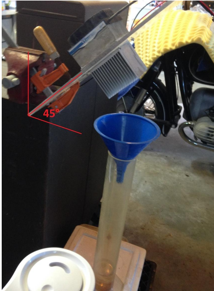
Figure 42. Tilted heatsink through flow experimental setup with 45° tilt.
