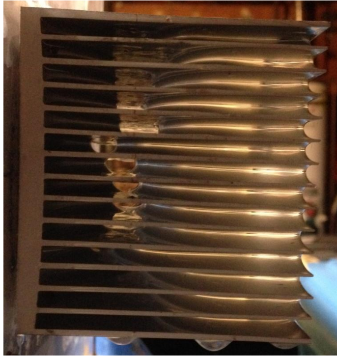
Figure 46. Tilted heatsink through flow condensate bridging at 90° (12 Hr).
