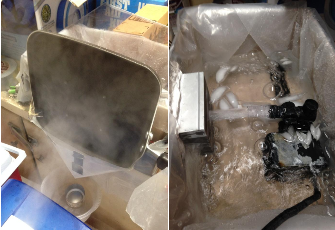
Figure 34. Water cooled TEC prototype experimental setup.
