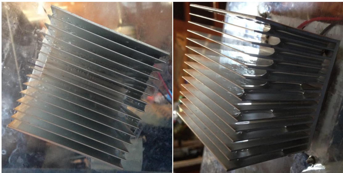
Figure 39. Tilted heatsink split flow condensate bridging at 60°.
