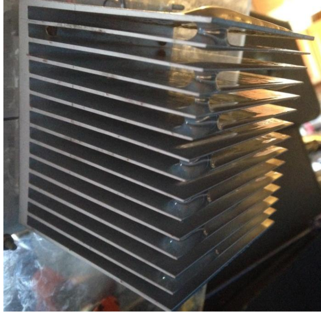
Figure 44. Tilted heatsink through flow condensate bridging at 60°.
