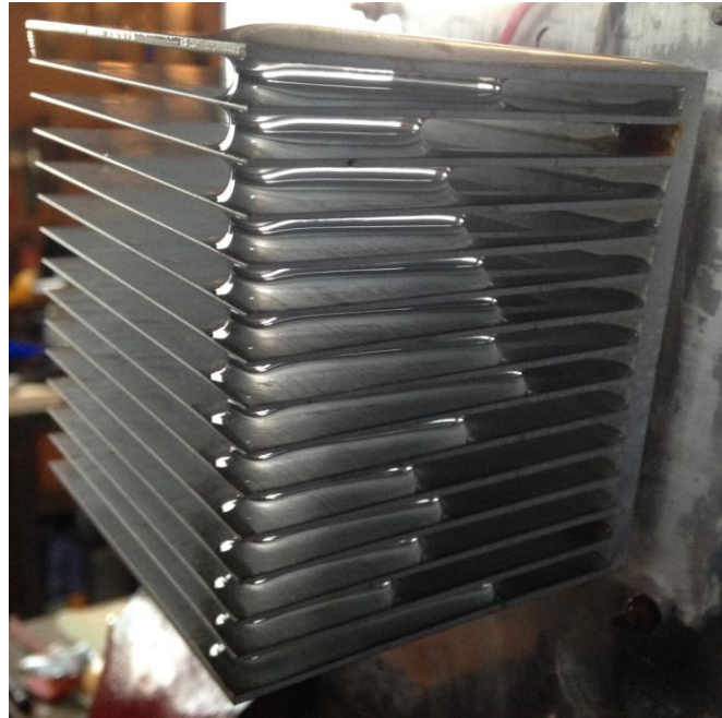
Figure 55. Tilted heatsink timeline condensate bridging at the 3 hour mark.
