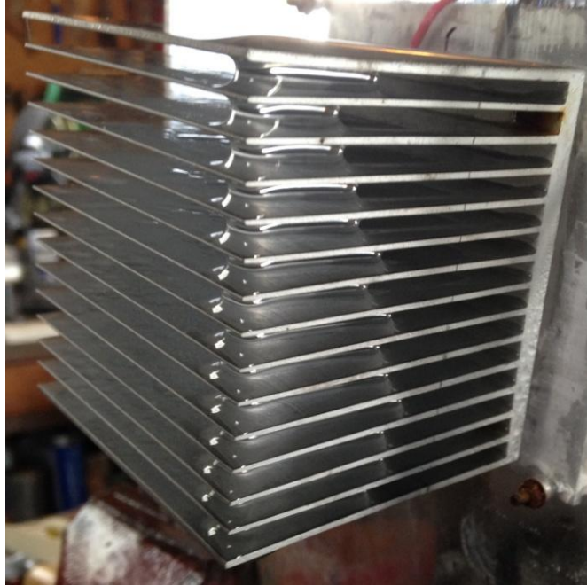
Figure 54. Tilted heatsink timeline condensate bridging at the 2 hour mark.
