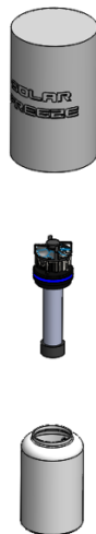
Figure 6. Exploded view of complete assembly. From top to bottom: Insulation Cover Assembly, Heat Transfer Assembly, and Vaccine Chamber Assembly.
