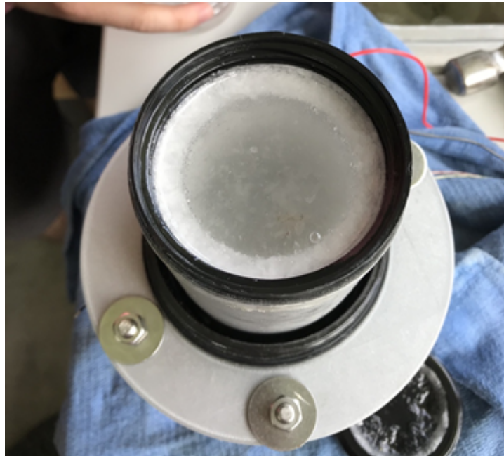
Figure 34. Partially frozen phase change material inside PCM container after 90 minutes of “charging”.
