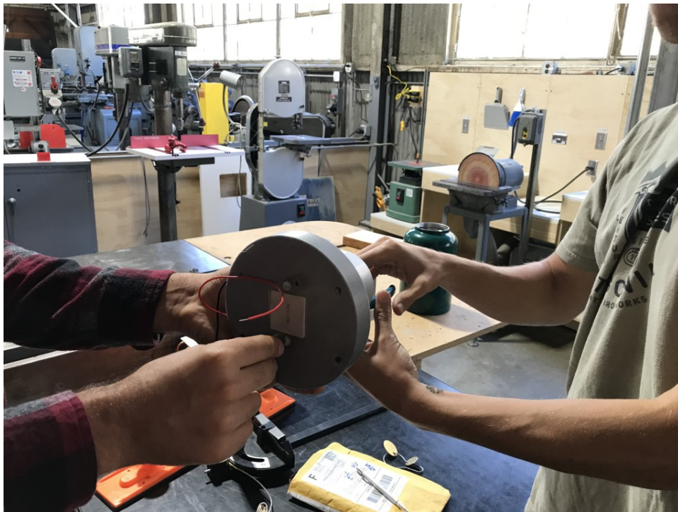
Figure 28. Attaching the cold side plate to the cap using nylon bolts.
