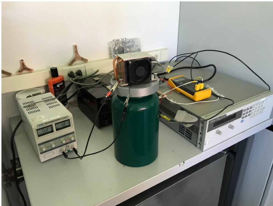
Figure 31. Freezing or “charging” testing configuration setup with fan/heat sink system and Peltier connected to power supplies.
