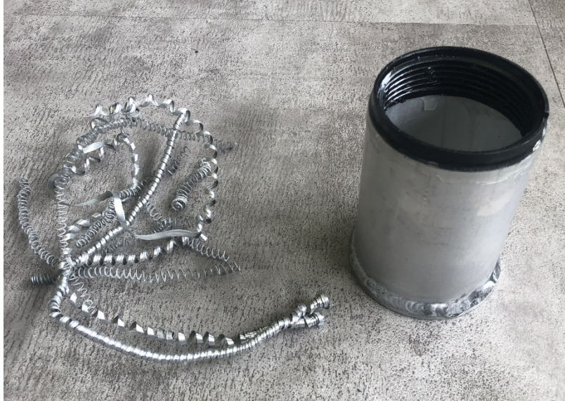
Figure 29. PCM container with aluminum metal shavings from a lathe.
