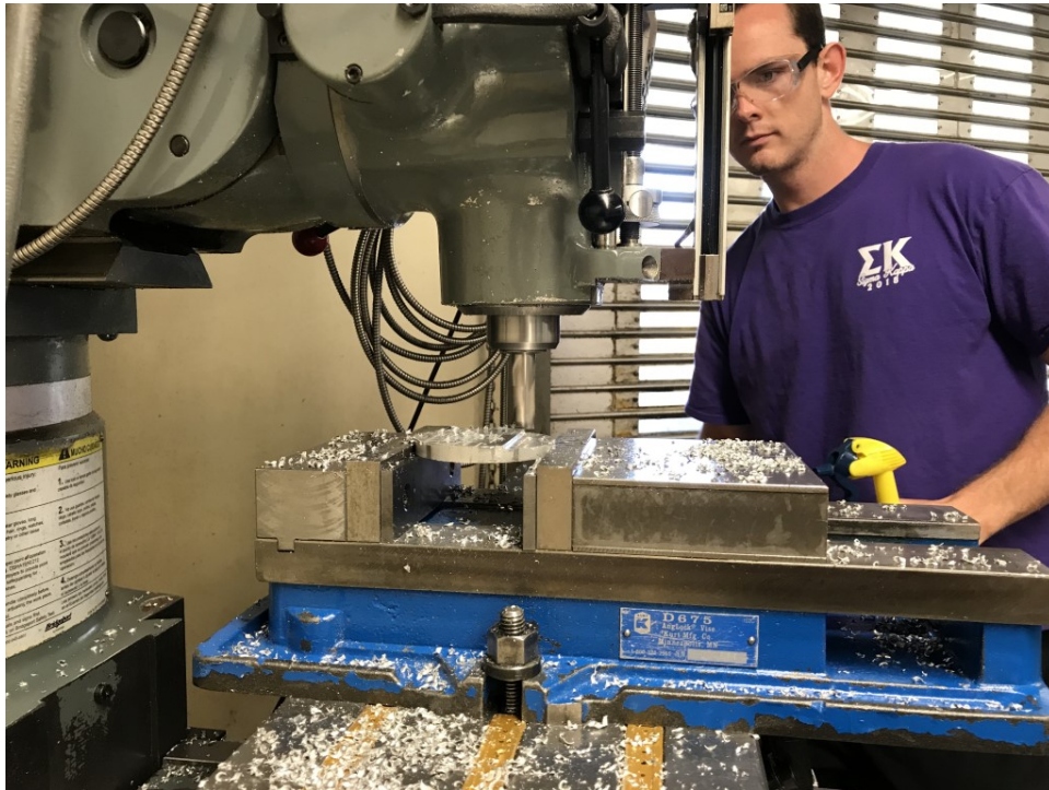
Figure 24. Solar Freeze team member Cody Volk using the mill to precisely trim down the thickness of the aluminum cold side plate.
