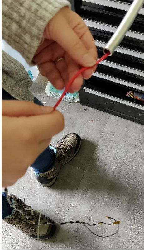
Figure 6. Beginning to put the diode chain through the tubing
