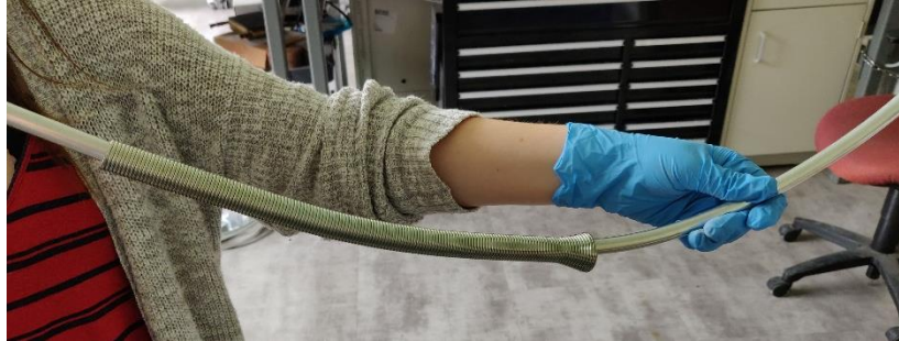
Figure 12. Putting the pipe bender onto the tubing
