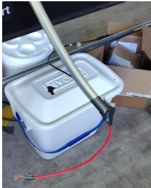
Figure 21. End of tube taped closed to prevent mortar leakage
