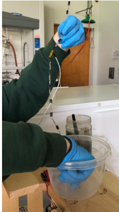
Figure 22. Feeding diode chain and mortar through pipe using manufacturing jig
