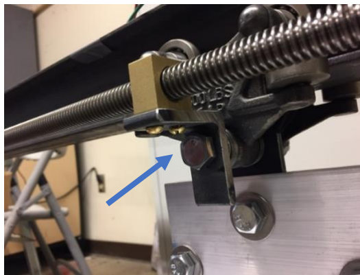
Figure 28. Trolley bracket connecting the lead screw nut to the trolley.
