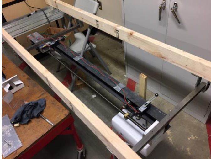
Figure 34. Assembled recumbent trike transfer device mounted to mock ceiling joists.
