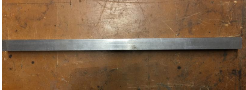
Figure 25. Carbon steel support beam cut to length.
