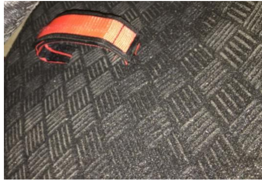
Figure 32. Velcro foot strap threaded through garage mat for foot securement.
