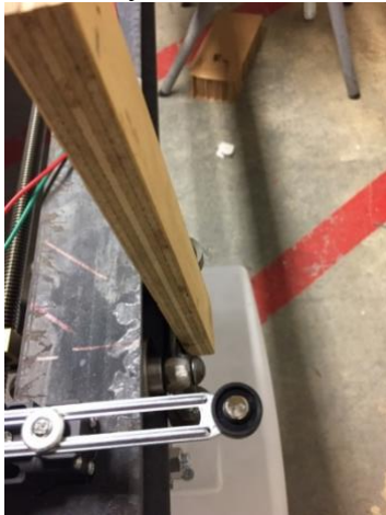
Figure 31. Limit switch trigger, initially a piece of plywood, but later replaced by a Simpson Strong-Tie steel piece.
