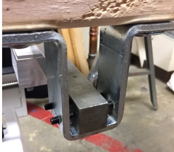
Figure 30. U-bracket, fixes to support beams using four set screws. A bolt set through the support beam end was added later to ensure the support beam does not slide out of the bracket.
