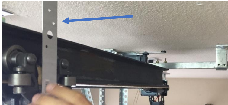
Figure 31. Limit switch trigger, initially a piece of plywood, but later replaced by a Simpson Strong-Tie steel piece.
