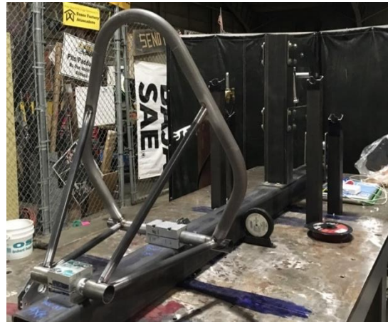
Figure 66. Roll hoop and rear triangle set up, using tube blocks to locate for wheel spacing, as built.
