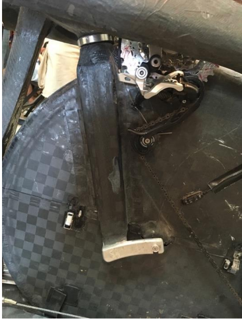
Figure 2. Picture displaying Eta Prime's fork offset.
