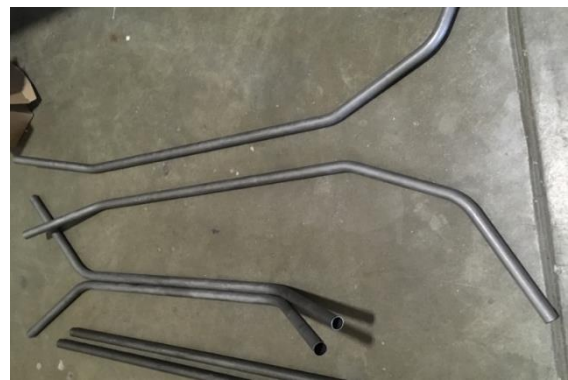
Figure 62. The middle side supports and top side supports, bent by Advance Tube.
