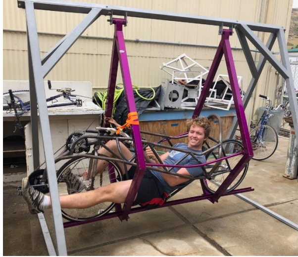
Figure 102. Josh Gieschen on the frame in the radius of gyration testing swing.
