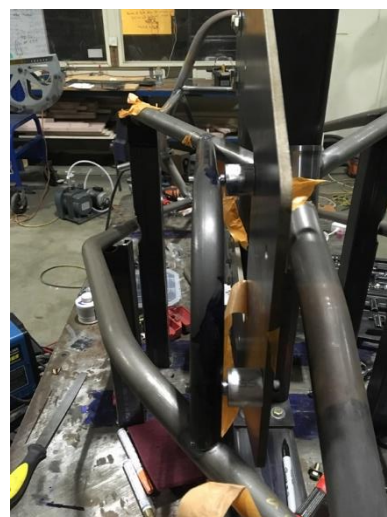
Figure 73. Jigging for mid drive truss, as built.
