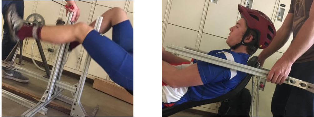
Figure 46. Testing with physical gauges around potential pinch or hazard points of the rider with frame or drivetrain.
