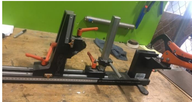
Figure 78. Anvil fork jig to be used in fork manufacture.
