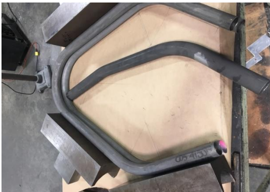
Figure 61. Bottom bracket support, roll hoops, bent by Advance Tube.
