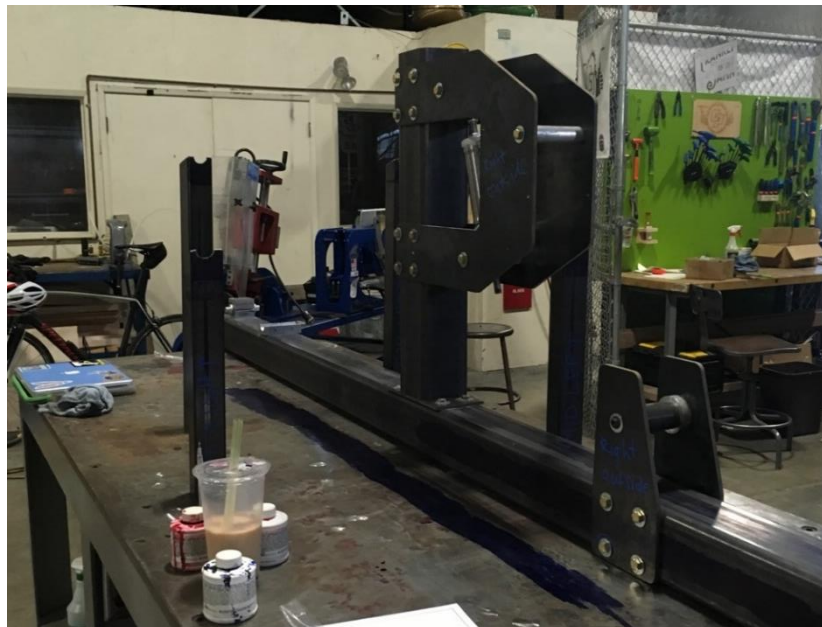
Figure 64. Overall first stage frame jig assembly, as built.
