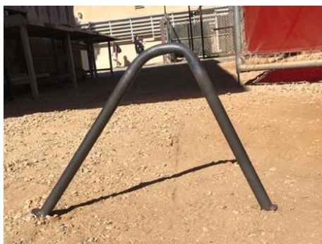
Figure 141. Hot Worked bending on homemade die.
