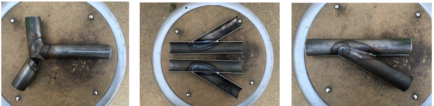
Figure 96. Left to Right: 90-degree sample, showing base metal failure; 30-degree sample, cross section showing full penetration; 30-degree sample, top view.
