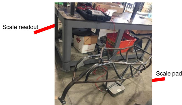
Figure 99. Setup for weighing of the frame.
