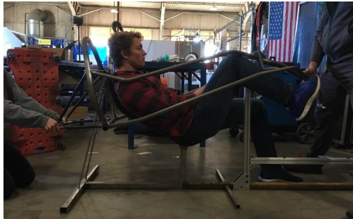
Figure 82. Test fit with Josh, top half of the bike and Josh in rider testing jig.
