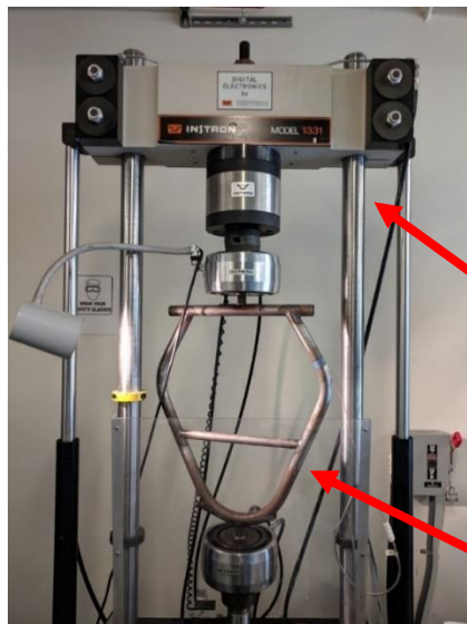
Figure 89. Vertical loading setup.
