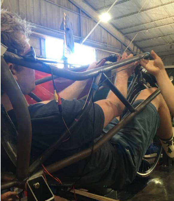
Figure 86. Third test fit with Josh, checking clearance on the shoulder truss members, with steering system and handlebars assembled.
