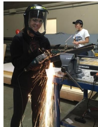
Figure 51. Keyanna Henderson using an angle grinder to cut a jig piece.
