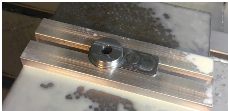
Figure 49. Second operation of front dropouts in softjaws on the Minimill.
