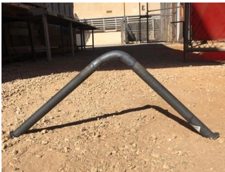
Figure 139. Hot Worked bending on homemade die.
