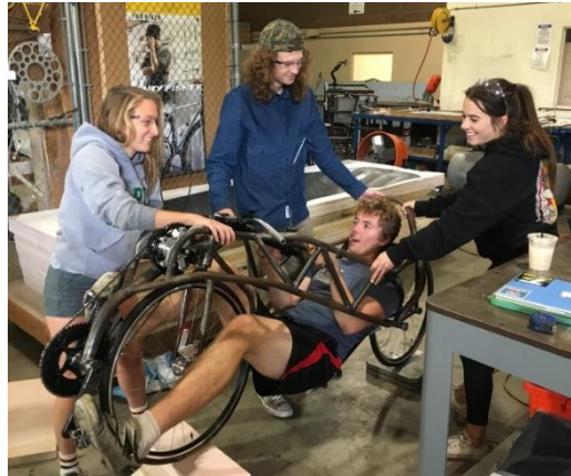
Figure 101. Inclined testing for center of gravity, with Josh in vehicle, and front wheel raised on foam blocks. Team members stand by to stabilize the vehicle.
