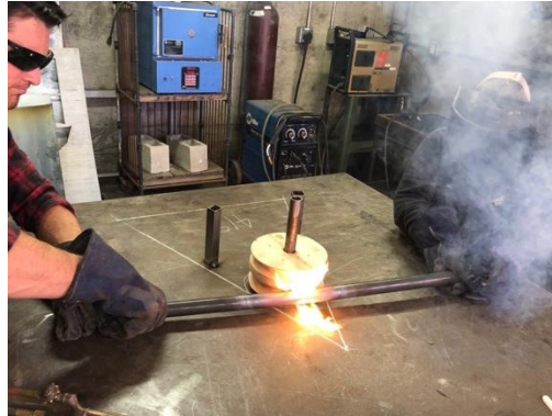
Figure 132. Hot worked bending on homemade die.
