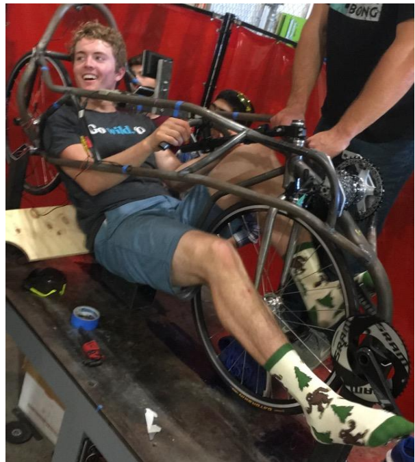
Figure 85. Test fit checking clearances with leg truss members, fork with wheel assembled, and final cranks on the vehicle. Vision system and mid-drive also assembled.
