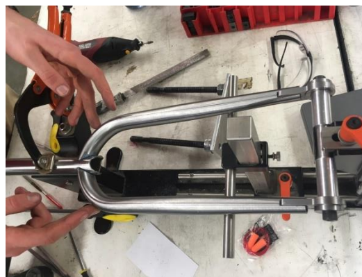
Figure 79. Fork assembled on fork jig, before welding, with steerer, front dropout, and custom dummy front axle.
