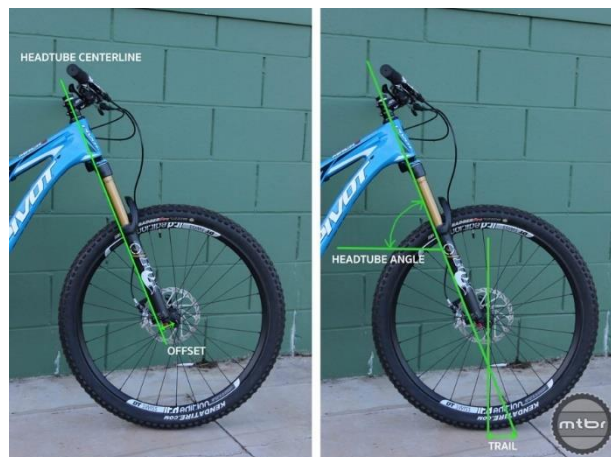
Figure 1. Graphic showing fork offset and trail [1].
