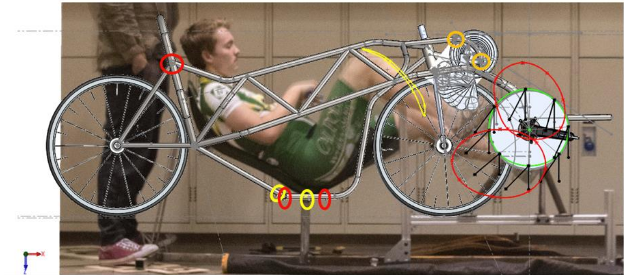
Figure 29. Overlay of frame with picture of rider, Josh, in testing jig set at final seat back angle and bottom bracket location.
