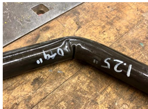
Figure 136. Bent tube showing failure by crinkling.
