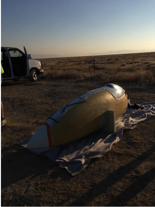
Figure 121. Kevlar fairing protector on IUT Anney's vehicle.
