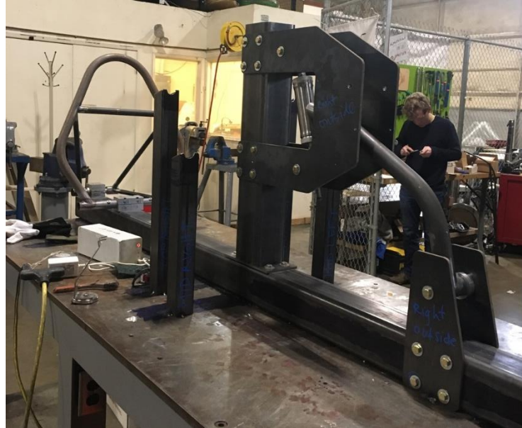
Figure 69. First stage frame jig with roll hoop, rear triangle, head tube, bottom bracket, and bottom bracket support located.
