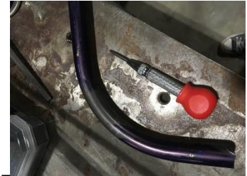
Figure 74. A marked and mitered mid drive truss, ready to drill.
