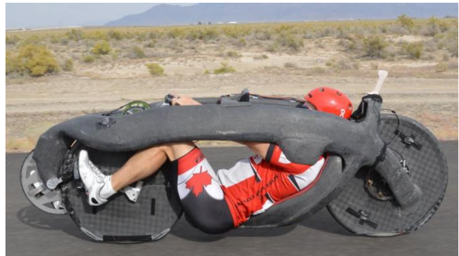
Figure 3. Eta with rider, showing the rider's position in the frame [6].
