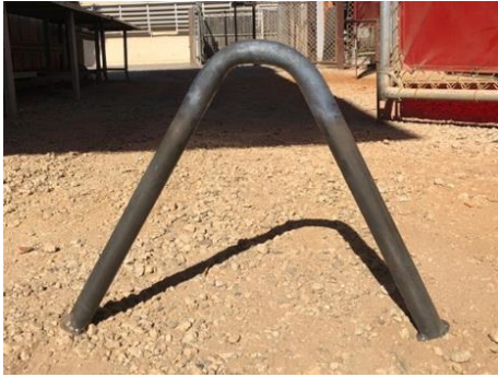
Figure 137. Hot Worked bending on homemade die.
