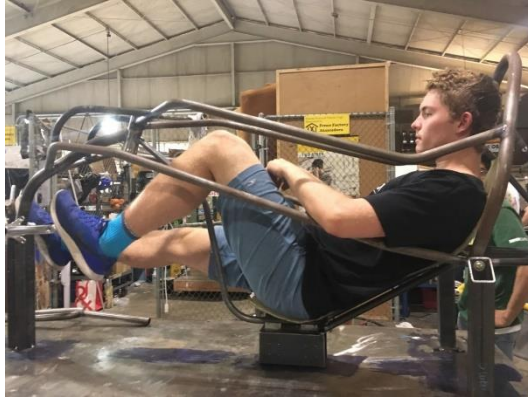
Figure 84. Second major test fit, side view, checking Josh's pedal circle clearance with the frame.
