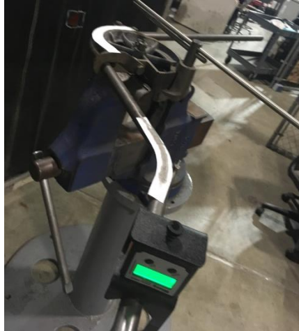
Figure 52. Set up of the bottom bent member on the bender.
