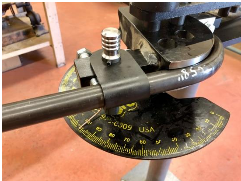
Figure 133. Cold worked bending on shop jig showing this tube was bent to 100°.
