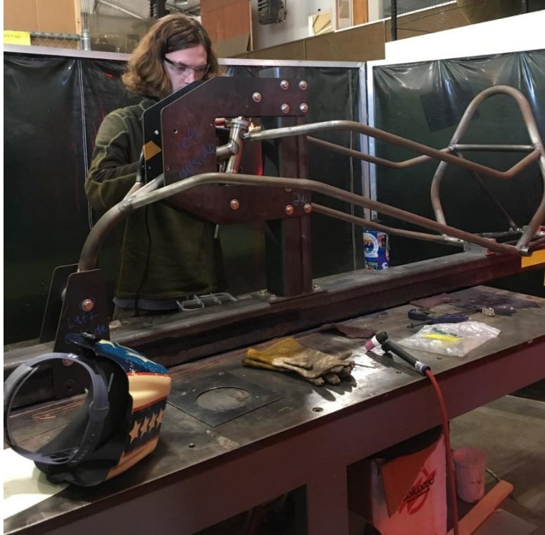
Figure 58. Eliot, the team welder, prepping joints for welding.
