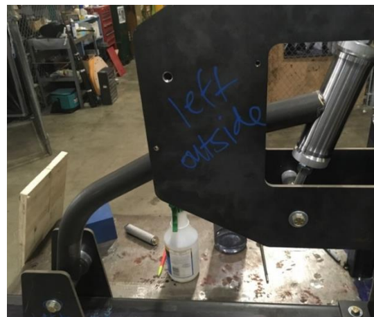
Figure 68. Front part of first stage frame jig, locating headtube and bottom bracket, as built.
