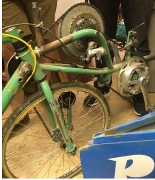
Figure 4. Primal 2's drivetrain and bottom bracket height in relation to the wheels.
