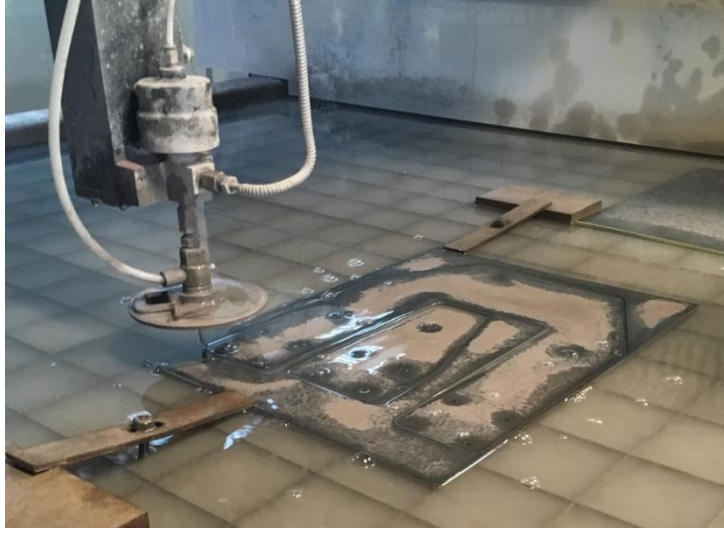
Figure 50. Top and Front plates being cut on the water jet.
