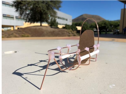
Figure 130. Frame with bottom and side bracing and side and back impact foam.
