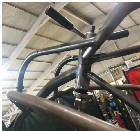
Figure 81. After post machining, pressing in bearing cups with headset press.
