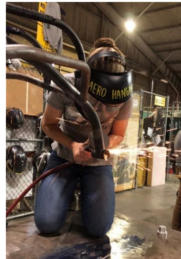
Figure 88. Kyra Schmidt cutting out the incorrect bottom bracket shell.
