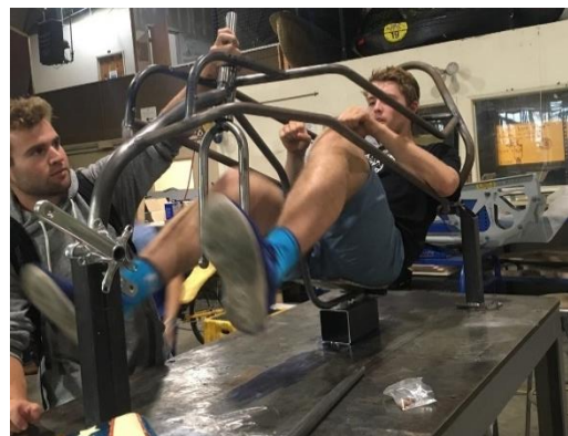
Figure 83. Second major test fit, with representative length cranks, fork, bottom members and seat.
