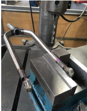
Figure 80. Fork boss set up on the drill press.
