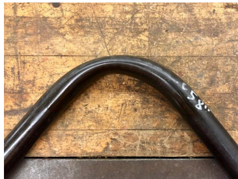
Figure 134. Bent tube showing failure by deformation.
