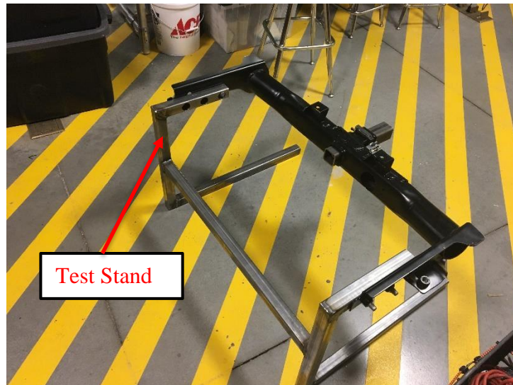
Figure 60: OEM Jeep hitch receiver mounted to receiver test stand.
