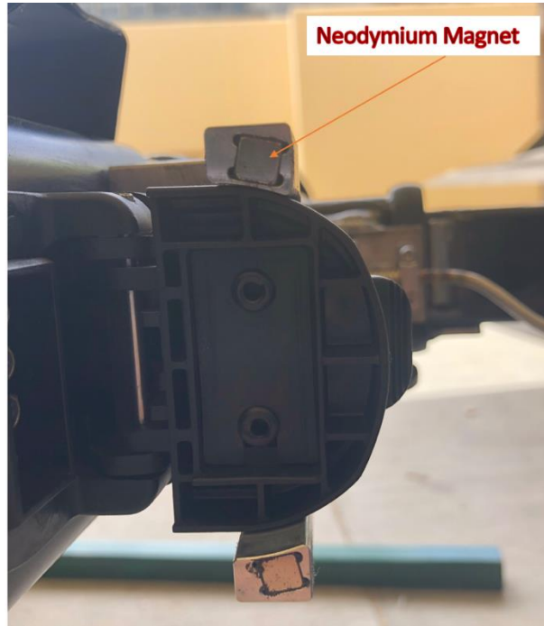
Figure 54: Neodymium magnets in the receptacle cage
