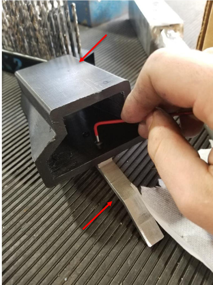
Figure 58: Securing the Incline to the Collar.
