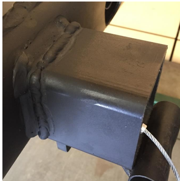
Figure 31: Receiver extension welded completely on
