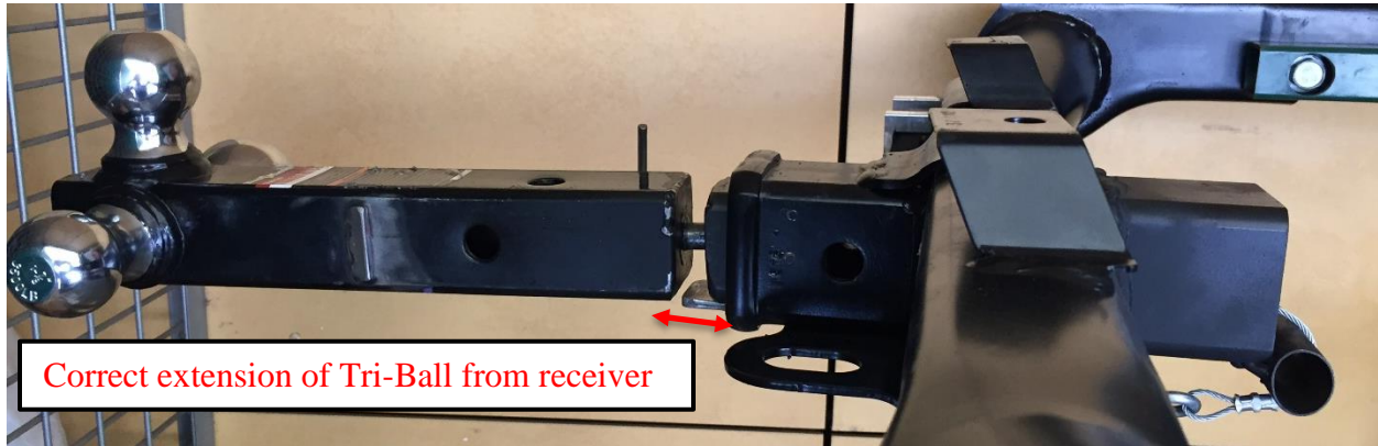
Figure 46: Proper cable length adjustment results in this maximum Tri-Ball hitch extension
