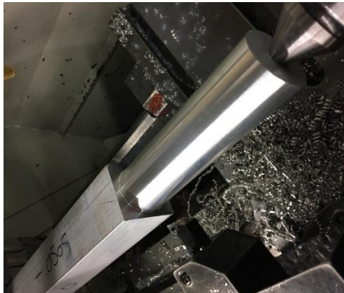
Figure 39: Turning the handle for the tongue lever
