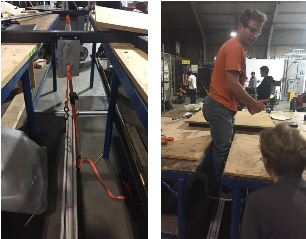
Figure 40. Load testing setup (left) and test in progress (right)
