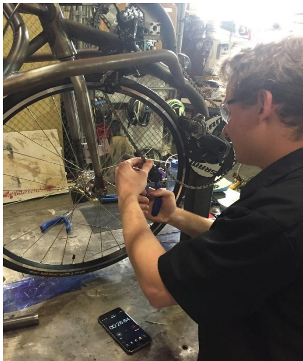
Figure 39. Chain installation time test
