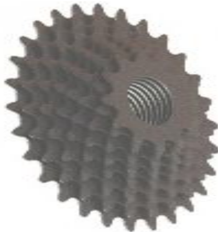
Figure 19. Modified 11 speed cassette with 8 gears ranging from 12-28 teeth
