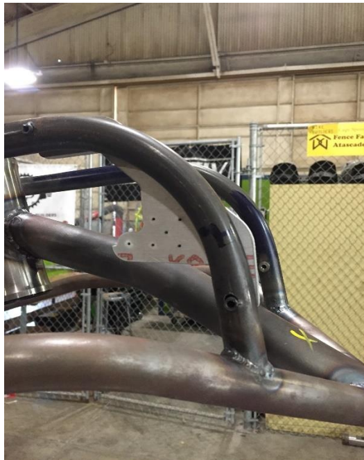
Figure 30. First-iteration fit test of right mounting plate on frame
