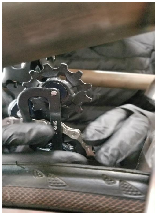
Figure R14. First Stage Chain Installation
