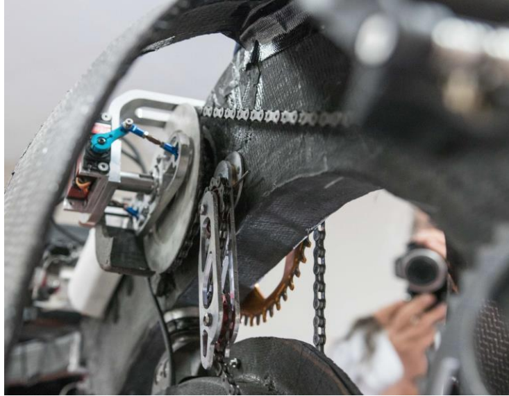
Figure 2. First-stage reduction of TU Delft’s drivetrain with electronically shifted cassette
