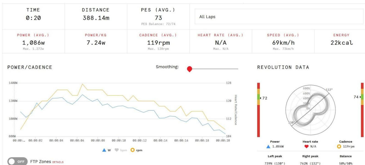
Figure A2. Eric - Sample Rider Power Data (20 second power sprint test)
