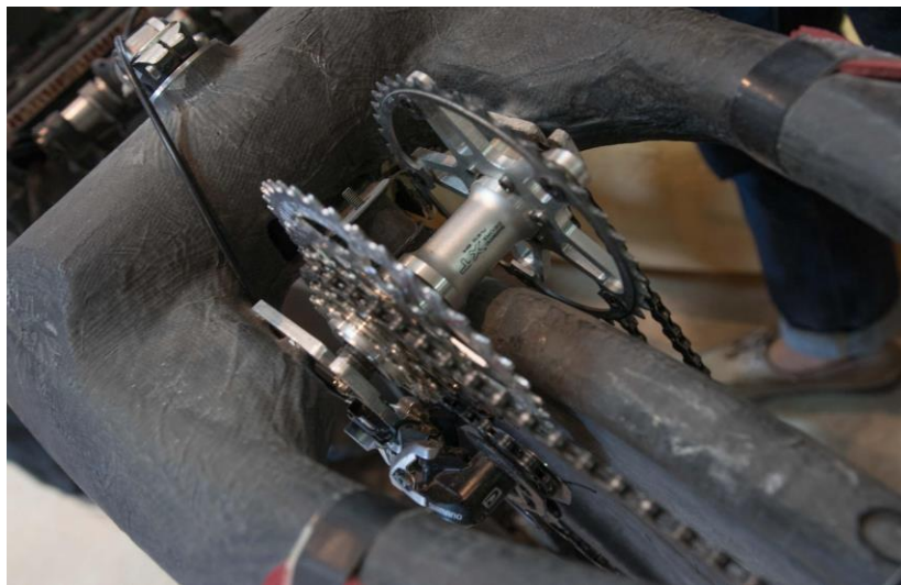
Figure 3. University of Toronto’s mid-drive with a 4-Gear cassette
