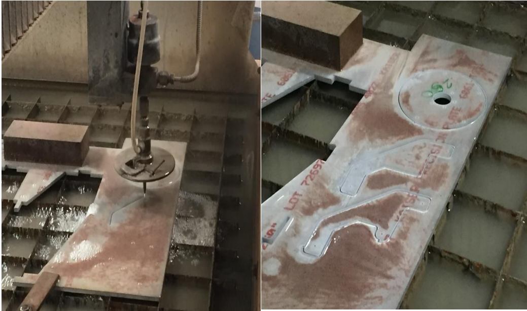
Figure 29. Waterjet outer profile and hole locations on mid-drive mounting plates and adapter
