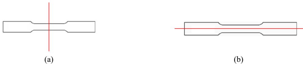
Figure 11. Diagram showing the cross-section (a) and longitudinal (b) cuts made on the stress rupture specimens received from PCC Structurals.
