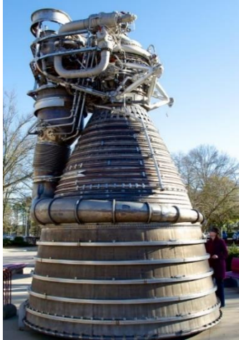
Figure 1: Image of the F-1 rocket engine, capable of producing 1.5 million pound-force of thrust and standing 18.5 feet tall 1 .
