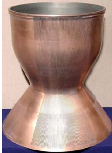
Figure 4: Main combustion chamber manufactured from GRCop-84 using vacuum plasma spraying. The converging-diverging conical shape allows for an increase of thrust and is typical of rocket engine exhaust geometry 4 .
