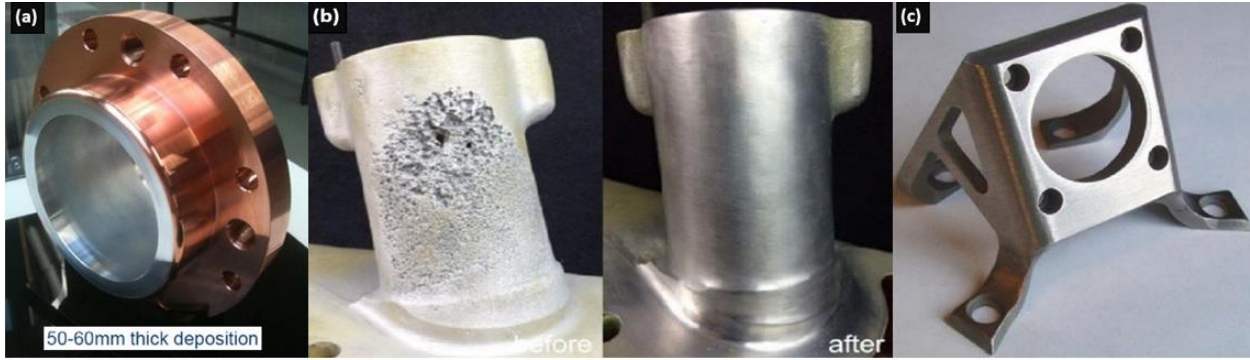
Figure 6: Example of cold spray in application for coating(a), repair(b) and additive manufacturing(c) 8 .
