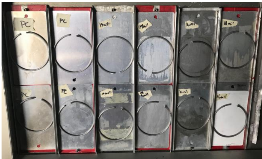
Figure 5. Samples placed inside the Q-U-V in a manner as to block as much radiation as possible.
