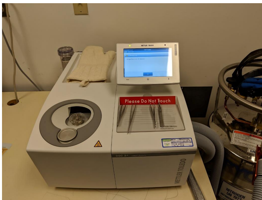
Figure 7: DSC3+ machine made by Mettler Toledo. The sample is put inside a crucible which is put on the stage at the left. The liquid nitrogen cooling inlet can be seen on the right.
