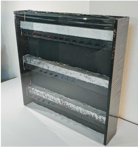
Figure 14. Concept prototype showing placement of bars and LEDs
