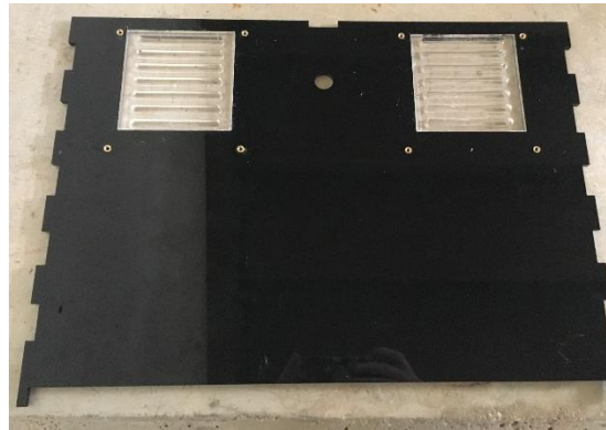
Figure 27. Thermal inserts in top sheet.
