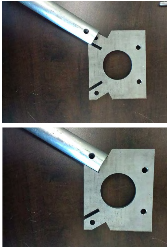
Figure 3. Sliding rear leg on rear plate.
