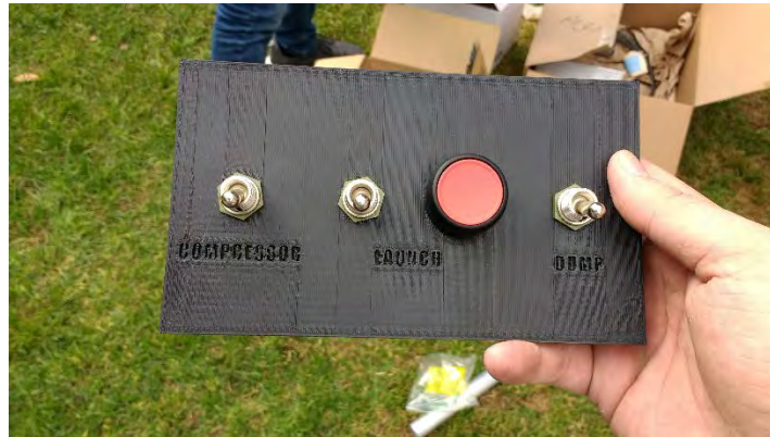
Figure 24. 3D printed launcher panel with switches installed
