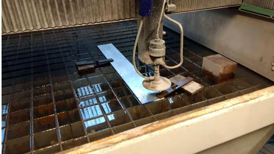
Figure 19. Water-jetting carriage components
