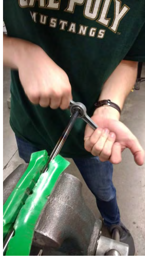
Figures 22 and 23. Pseudo-annealing and cutting threads on linear motion shafts
