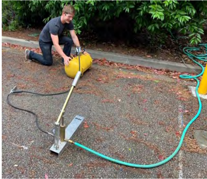
Figure 25. Hydro-testing pressure vessel and fittings
