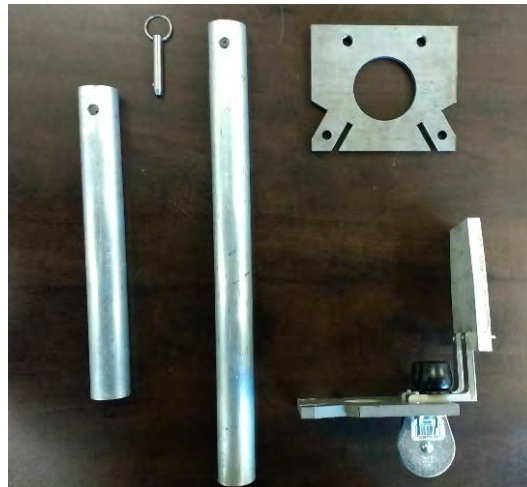
Figure 6. Front and back leg, front and back plate, quick release pins.
