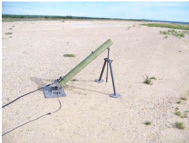
Figure 3. SeaCorp™ Inflator Based Launcher (Inflator-Based UAV Launchers)
