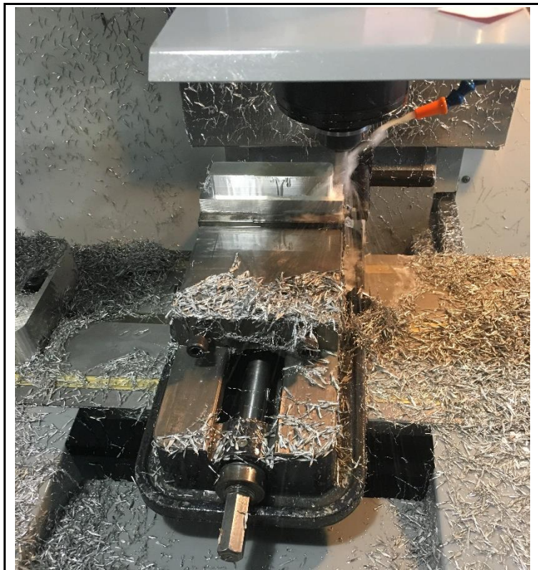
Figure 22 – Contour during the first operation on an aluminum boss.
