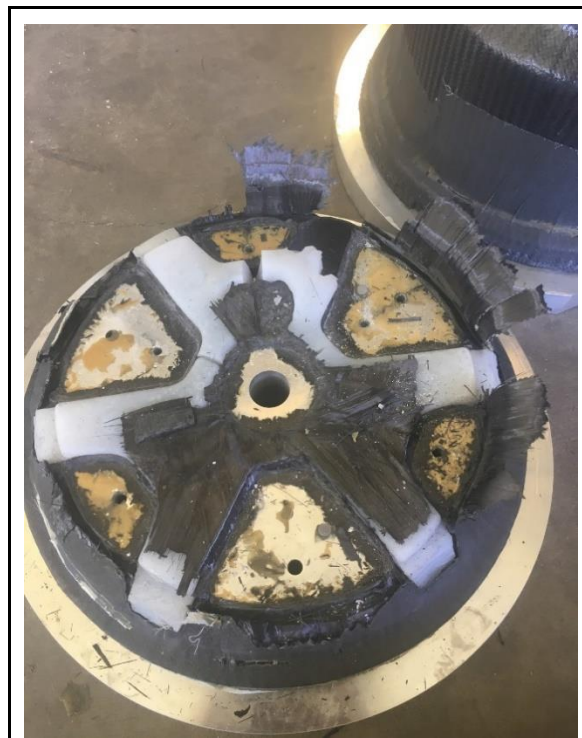
Figure 3 – Reinventing the Wheel's attempt to separate wheel from their mold.
