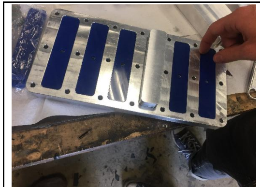
Figure 31 – Plastic shims used to define the process gap.
