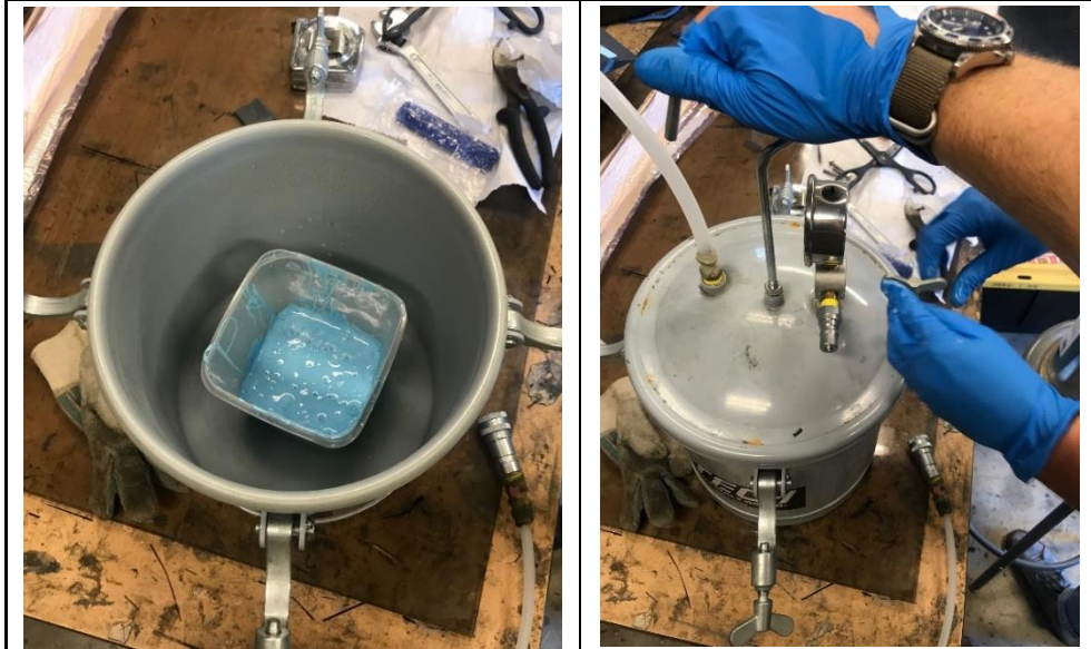
Figure 34 – Mixed silicone in the degassing chamber (left) and with the chamber being depressurized (right).
