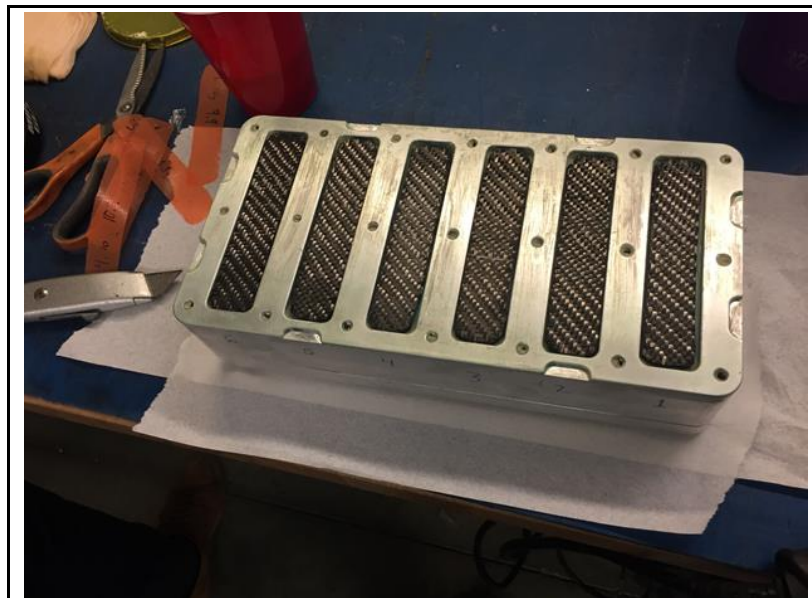
Figure 37 – Prepreg carbon fiber in the test coupon mold.
