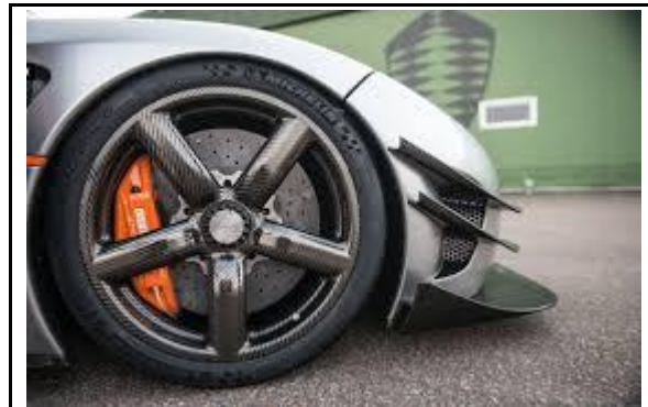
Figure 4 – Completed Koenissegg carbon fiber reinforced epoxy wheel.
