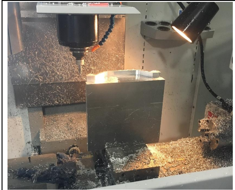
Figure 27 – Female mold setup for job operations two and three.
