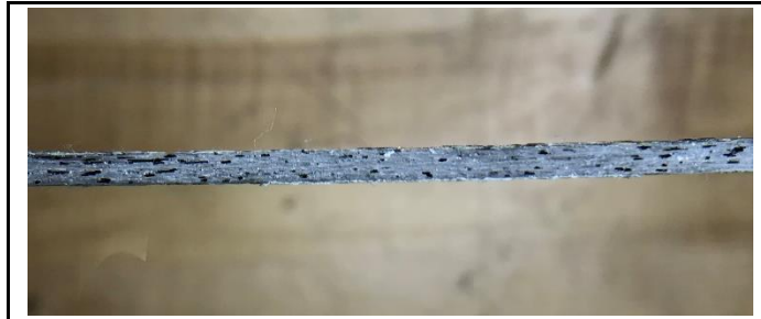
Figure 40 – Coupon Cross section: 1/16 in. process gap, insufficient compaction, formation of voids
