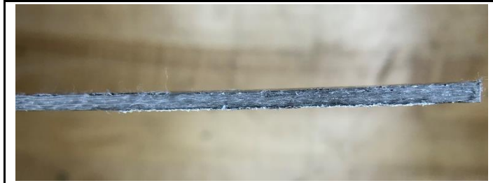
Figure 42 – Coupon Cross section: 1/16 in. pre-compaction, Resin over-bleed and poor bonding
