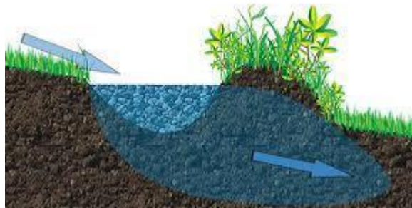
Figure 2. Diagram of the basic functionality of a swale. [6] Manufactured variations of swales exist for water collection and could potentially be employed in the Gravity Drip System for stormwater collection as is done in the patent for ‘ Elevated Swale... ’ [7].
