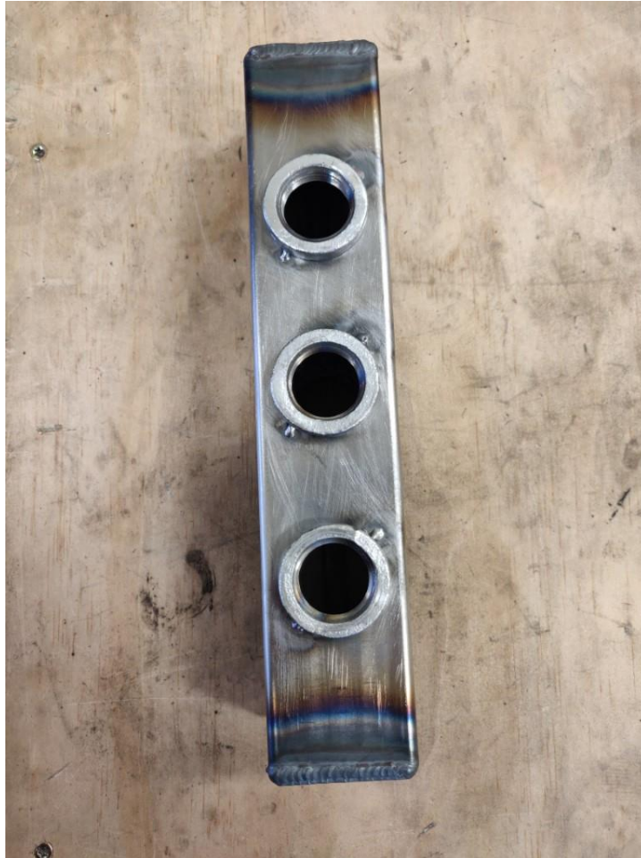
Figure 29. Manifold with located and tacked weld bungs.
