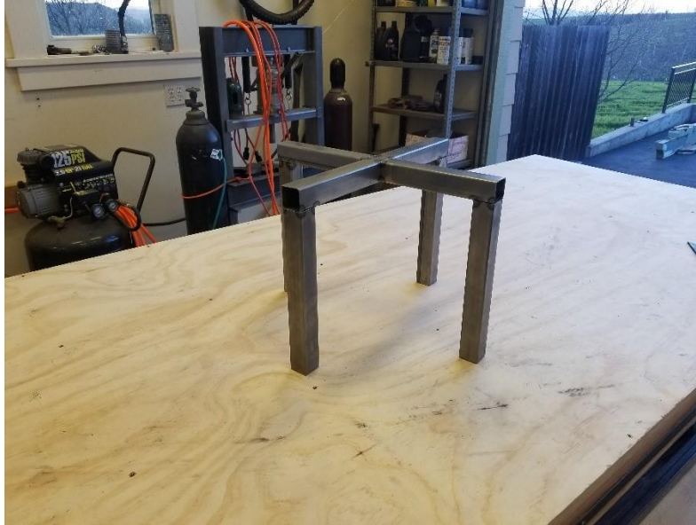
Figure 25. Cross frame with welded leg supports.
