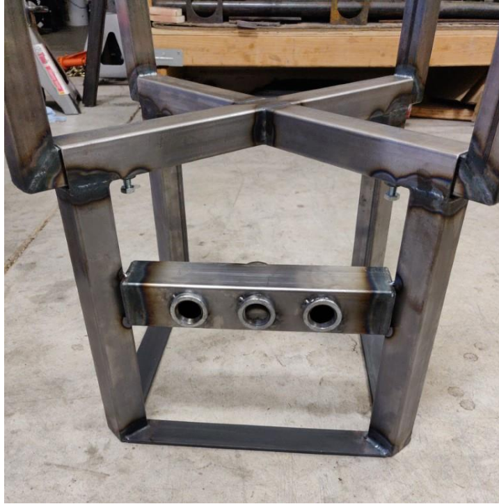
Figure 30. Fully welded frame assembly.
