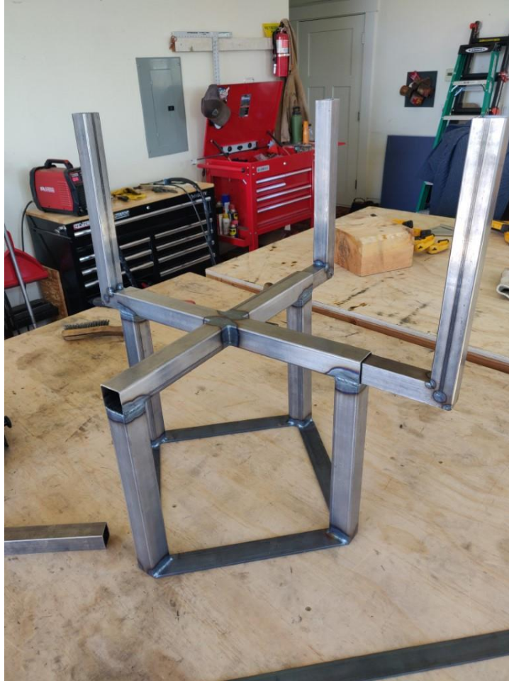
Figure 28. Welded base frame with telescoping arms inserted.
