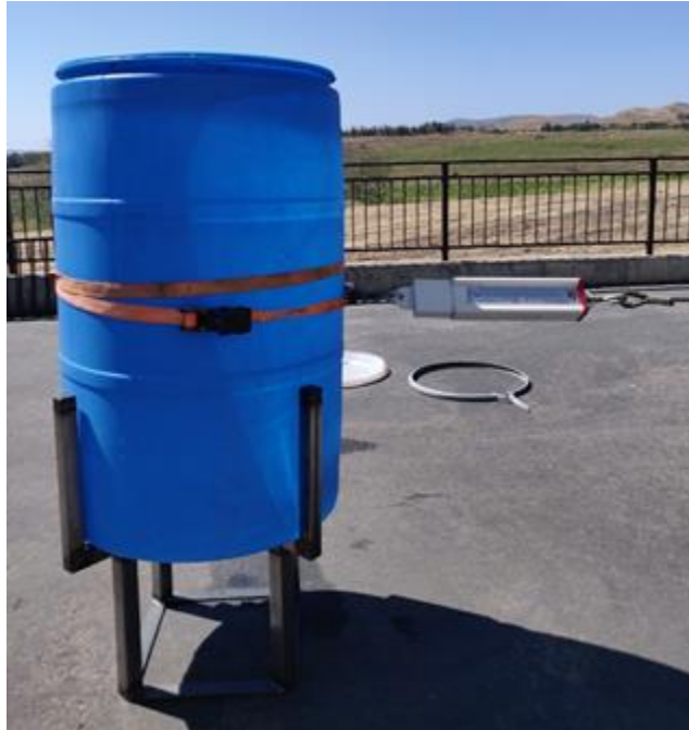
Figure 31. Water loaded barrel with attached load scale.
