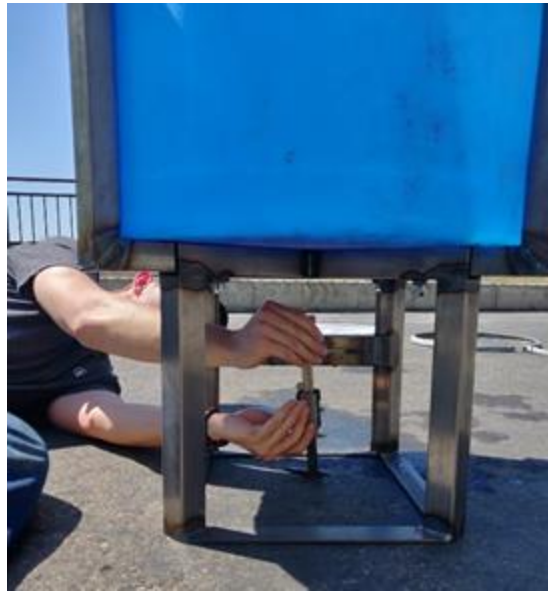
Figure 32. Preparing digital calipers to measure frame displacement under load.
