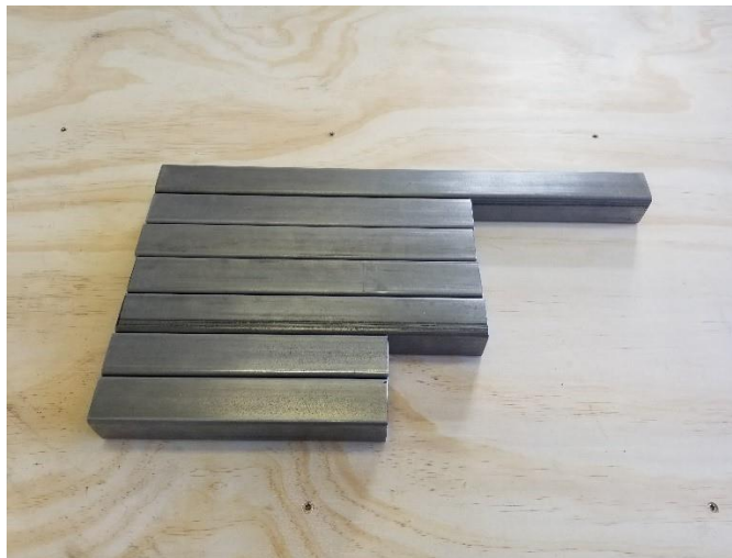
Figure 23. Cutting of system cross frame and legs to their appropriate lengths.
