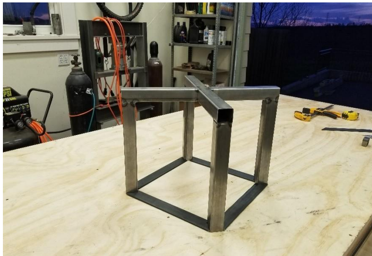
Figure 26. Frame with welded leg brackets.
