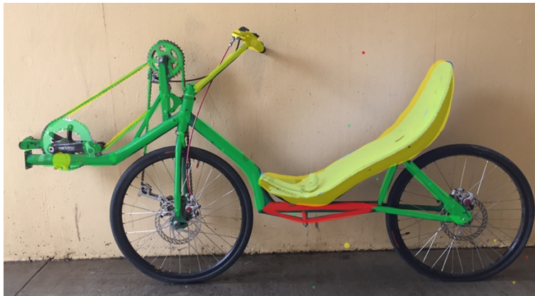
Figure 4. Portions of the primal 1 bike that will be removed, modified or utilized as shown for the trainer – highlighted in red, yellow, and green, respectively.
