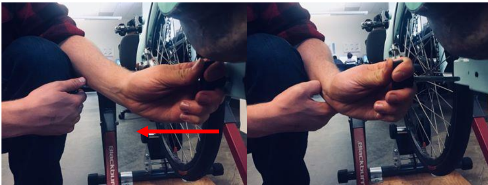
Figure 4. Proper Removal of Detent Pins
