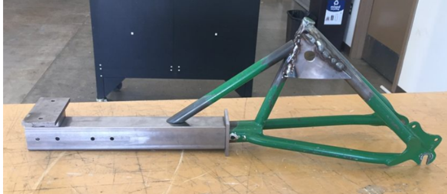
Figure 42. Finished back half of trainer frame – pre welding
