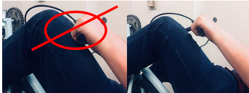
Figure 3. Ensure there is enough clearance between the handlebars and the rider's legs during operation
