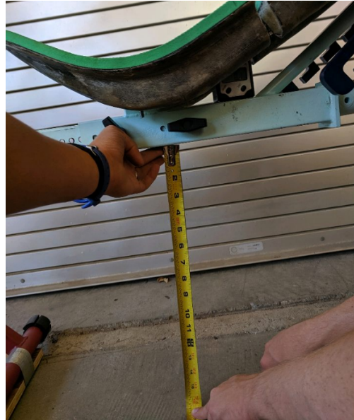
Figure 46. Measuring height of seat track at seat bolt location prior to load test
