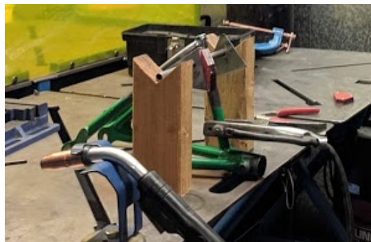
Figure 35. Rear triangle welding tabs – welding set up.
