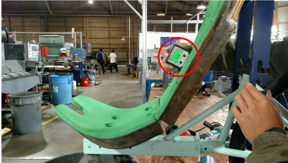
Figure 45. Seat back angle measurement verification test with angle gage
