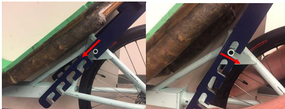
Figure 7: The motions required to remove the support arms from their current position
