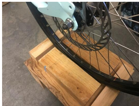
Figure 1. Back wheel properly secured in back support stand
