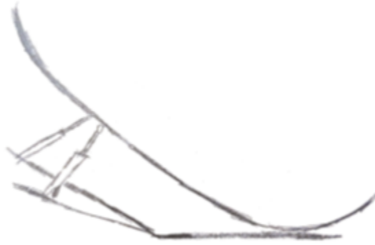
Figure 13. Seat back supported and reclined by two telescoping rods
