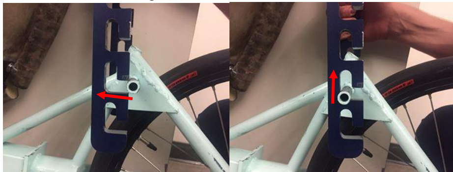
Figure 8. The motions required to secure the support arms at a new position
