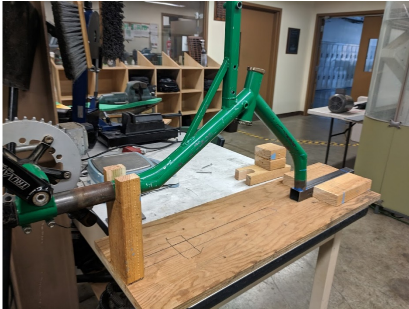
Figure 39. Front half welding jig with front half of Primal 1 and front box beam
