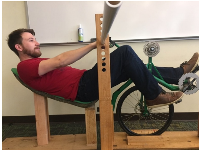
Figure 23. Structural prototype with participant and handlebar measurement device
