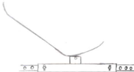
Figure 9. Seat track mechanism with spring-loaded pins and holes
