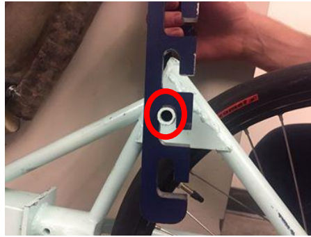
Figure 9. The final resting position of the support arms to ensure they are completely secured
