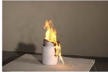
Figure 3.2-10. Trash container 2, 100 s after ignition
