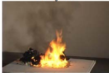
Figure 3.2-14. Trash container 2, 400 s after ignition
