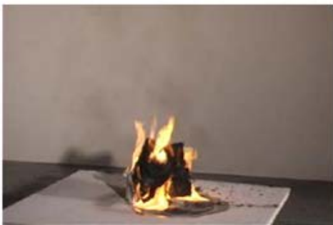
Figure 3.2-7. Trash container 1, 500 s after ignition
