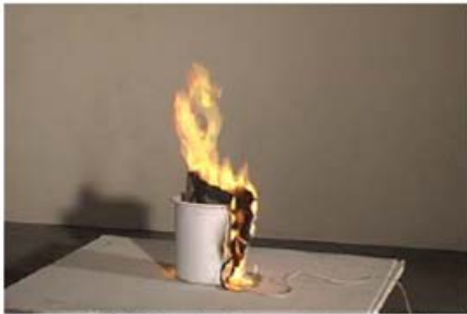
Figure 3.2-11. Trash container 2, 200 s after ignition
