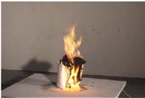
Figure 3.2-3. Trash container 1, 200 s after ignition
