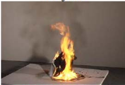
Figure 3.2-13. Trash container 2, at peak heat release rate, 363 s after ignition
