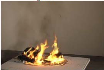
Figure 3.2-15. Trash container 2, 500 s after ignition
