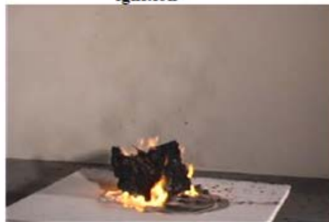
Figure 3.2-8. Trash container 1, 600 s after ignition
