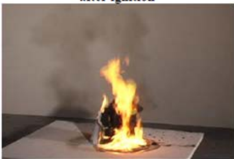
Figure 3.2-5. Trash container 1, 400 s after ignition
