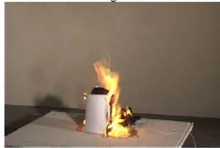
Figure 3.2-12. Trash container 2, 300 s after ignition
