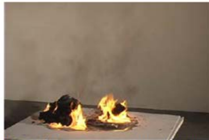
Figure 3.2-16. Trash container 2, 600 s after ignition
