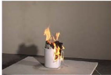
Figure 3.2-2. Trash container 1, 100 s after ignition
