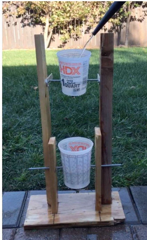
Figure C-2. Two-Bucket Testing Apparatus
