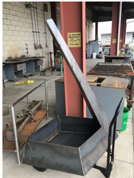
Figure 30. Lower Half of Fountain Welded
