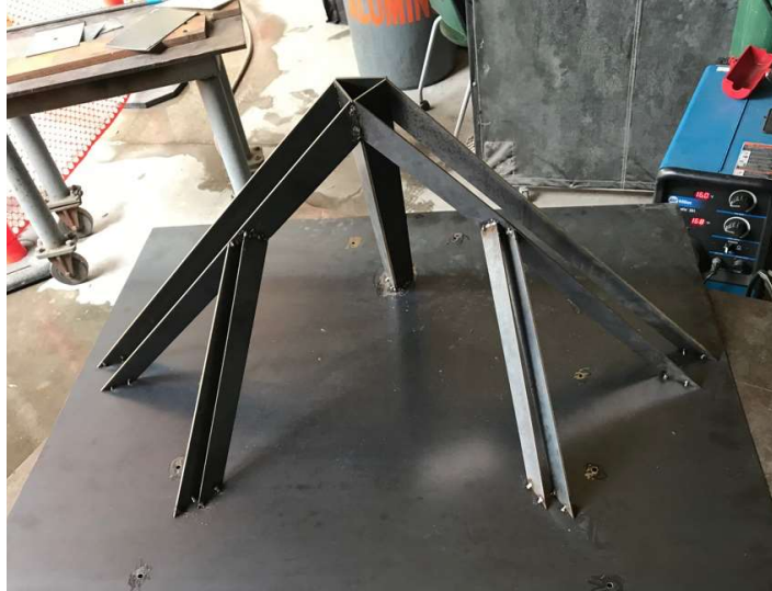
Figure 31. Top Half of Fountain with Welded Branches
