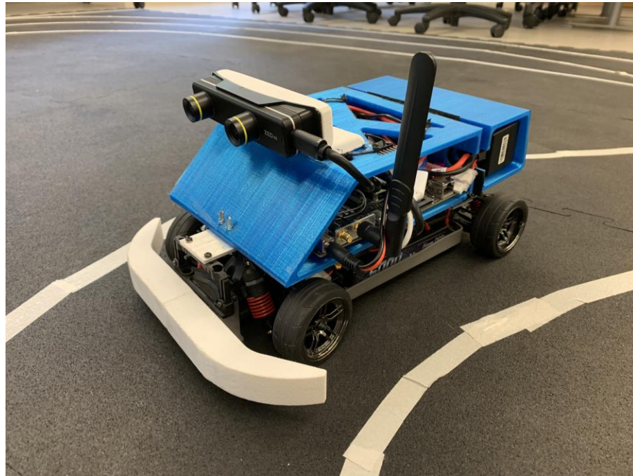
Figure 29. Final iteration of the car, with Zed Mini stereoscopic camera and final enclosures
