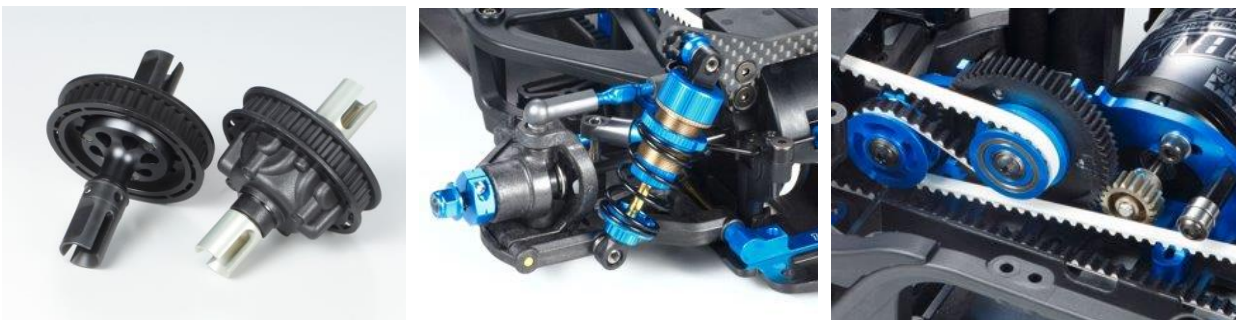
Figure 17. TA-07R Limited Edition featuring direct coupling and differential with aluminum gears, big bore damper and double wishbone suspension, and low-friction white belt (from left to right)
