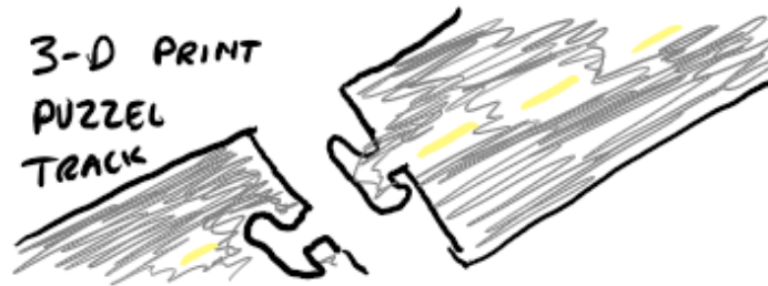
Figure 4: 3-D printed track that can be assembled like a puzzle and have interchangeable pieces
