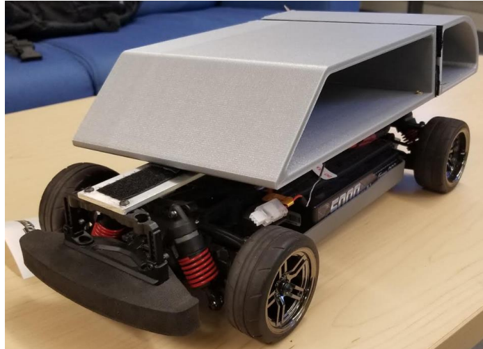
Figure 21. Isometric view with microcontroller housing and battery housing on Traxxas 4TEC 2.0 RC car. Velcro mounting is only temporary and used for purposes of this picture.
