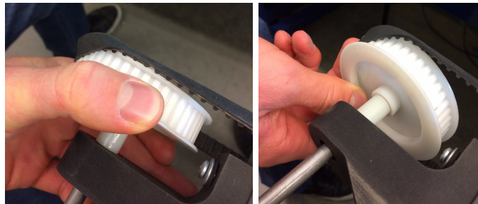
Figure 2. Cleaner Belt Installation on Flange
