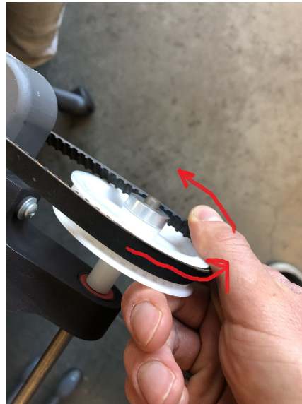
Figure 32. Belt Installation Process
