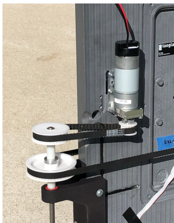
Figure 16. Motor Shaft to Bracket Shaft Linkage
