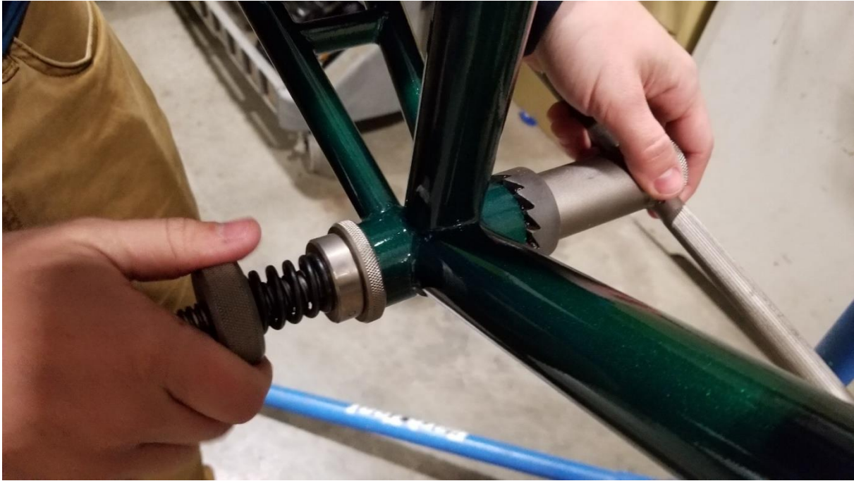
Figure 146. Facing the bottom bracket and chasing the threads
