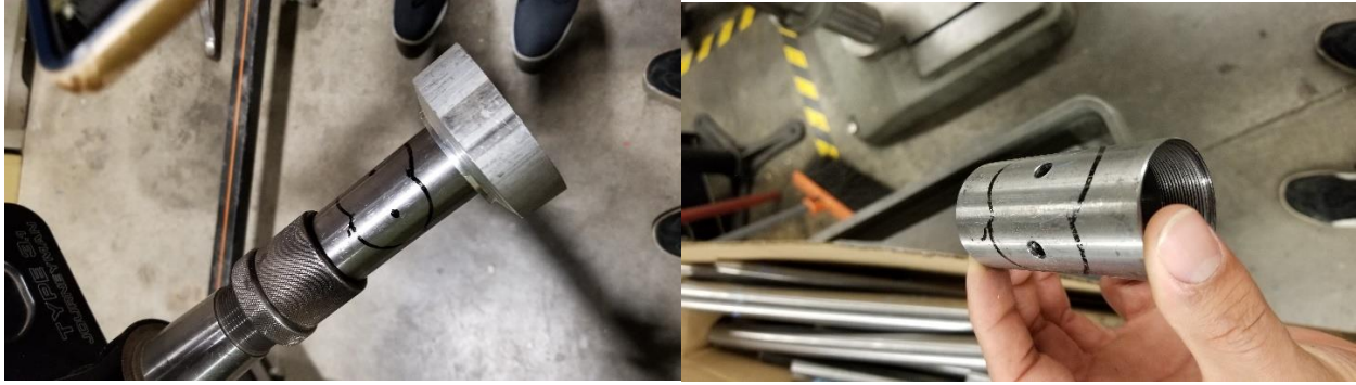
Figure 142. Example of the bottom bracket purge hole process
