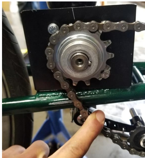
Figure 172. Demsontration of lack of chain wrap and chain tension in front driveetrian
