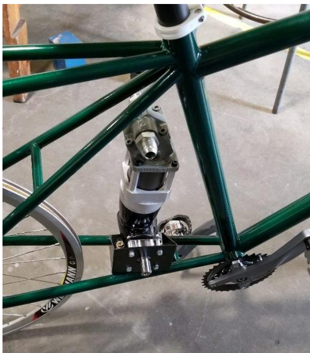
Figure 163. Planetary gearbox and pump attached to mounting bracket
