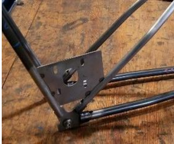
Figure 154. Rear drivetrain mount welded in place
