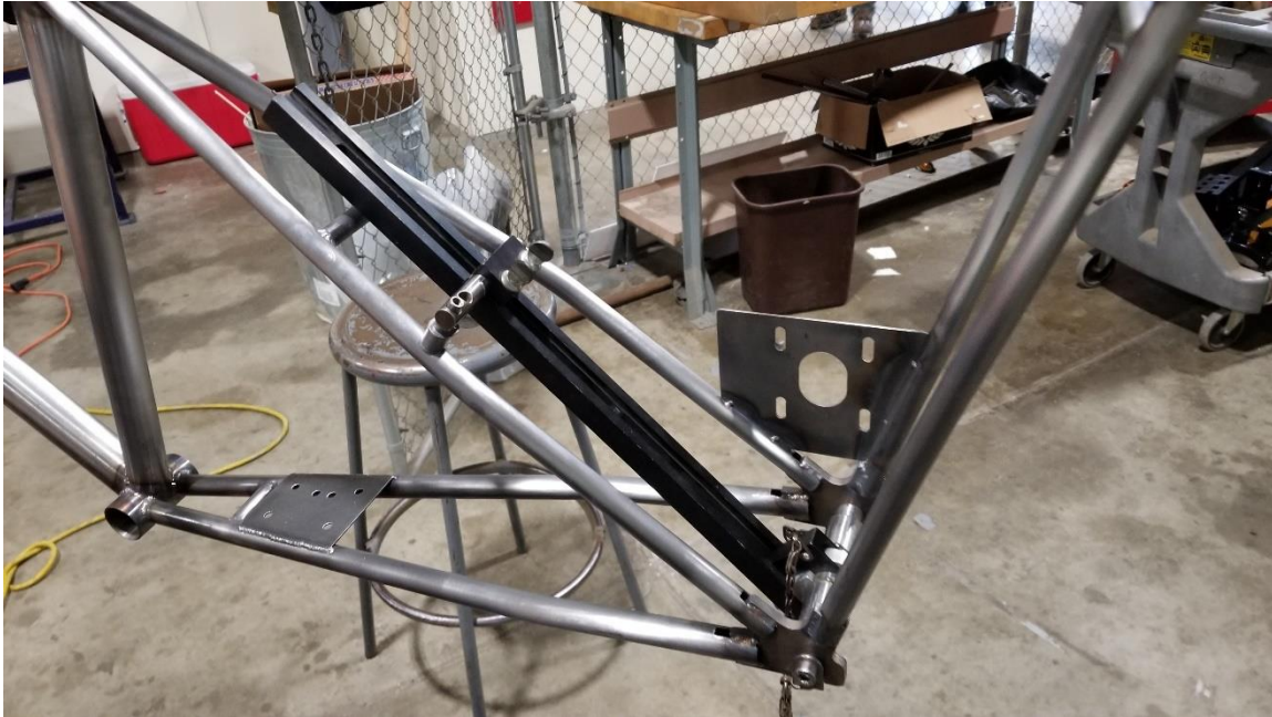
Figure 144. Image of rear brake boss brazing fixture attached to the rear dropouts
