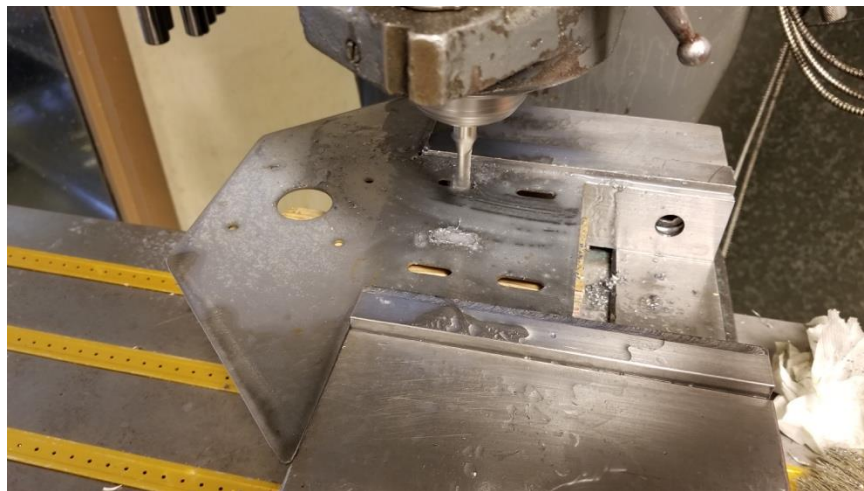
Figure 152. Machining additional slots into the front drivetrain mounting bracket using the mill in Mustang 60
