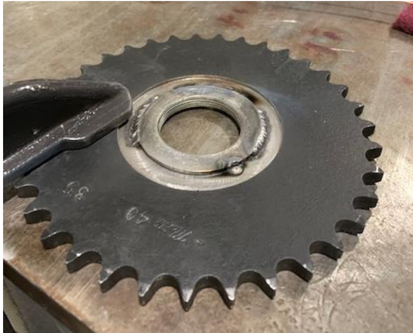
Figure 156. Rear fixie sprocket components welded together.
