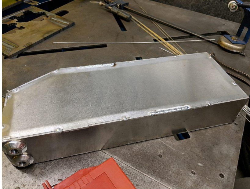
Figure 149. Final reservoir getting welded
