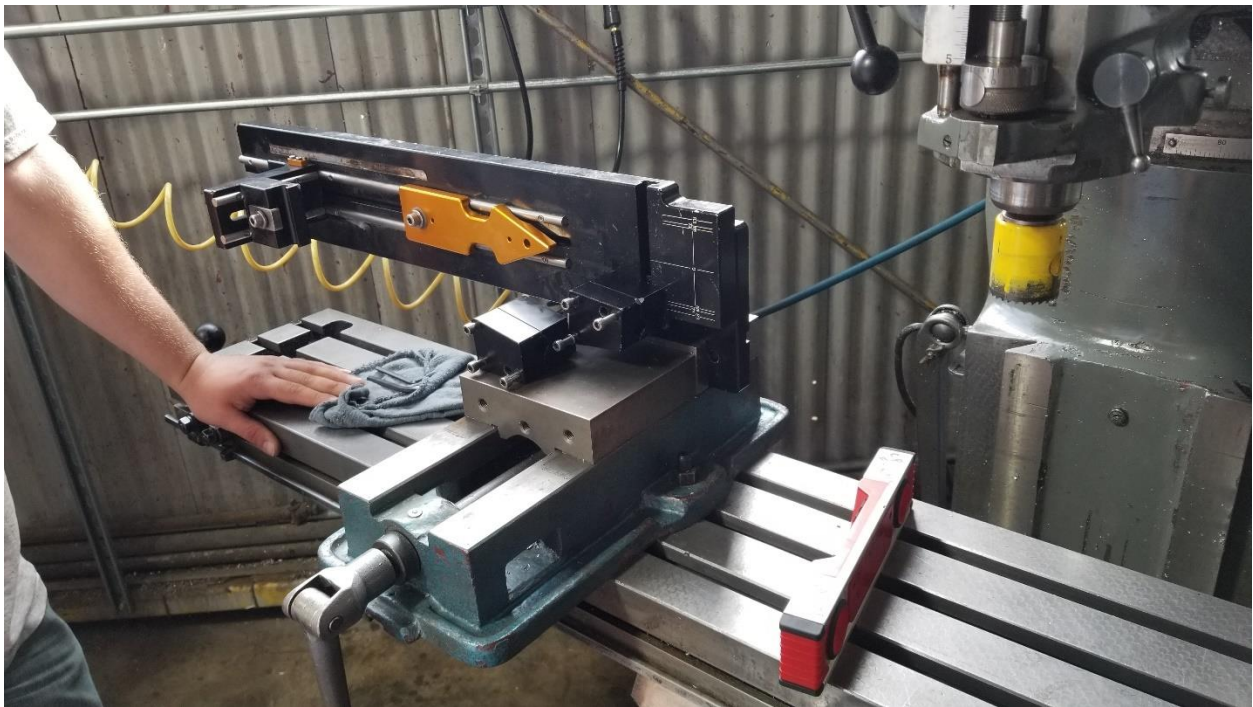
Figure 137. Another Anvil fixture used for the tubes attached to the bottom bracket
