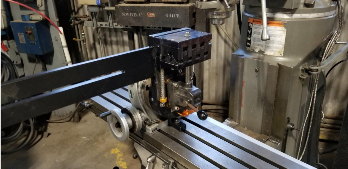
Figure 134. Anvil Universal Mitering Jig attached to a rotary vice on a mill
