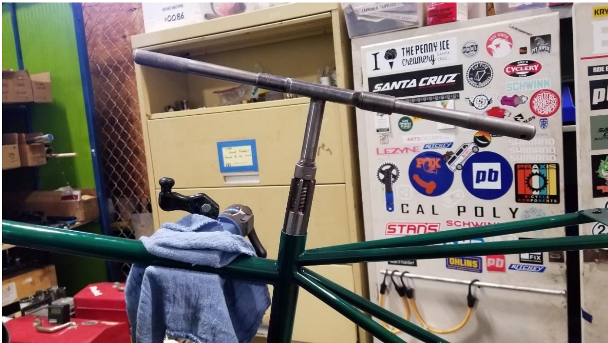
Figure 147. Reaming the seat tube
