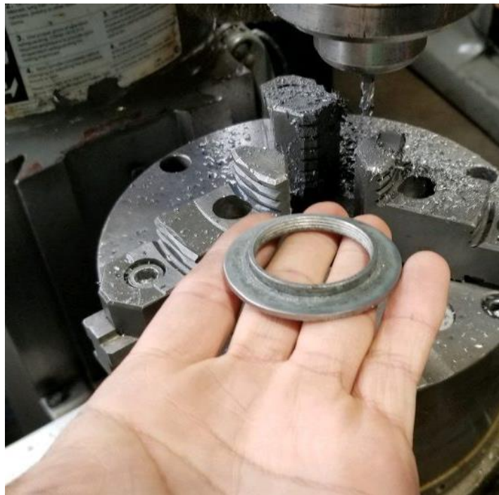
Figure 155. Fixie sprocket with teeth machined down
