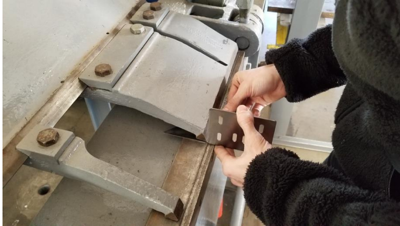
Figure 151. Bending the front drivetrain mounting bracket on the sheet metal brake
