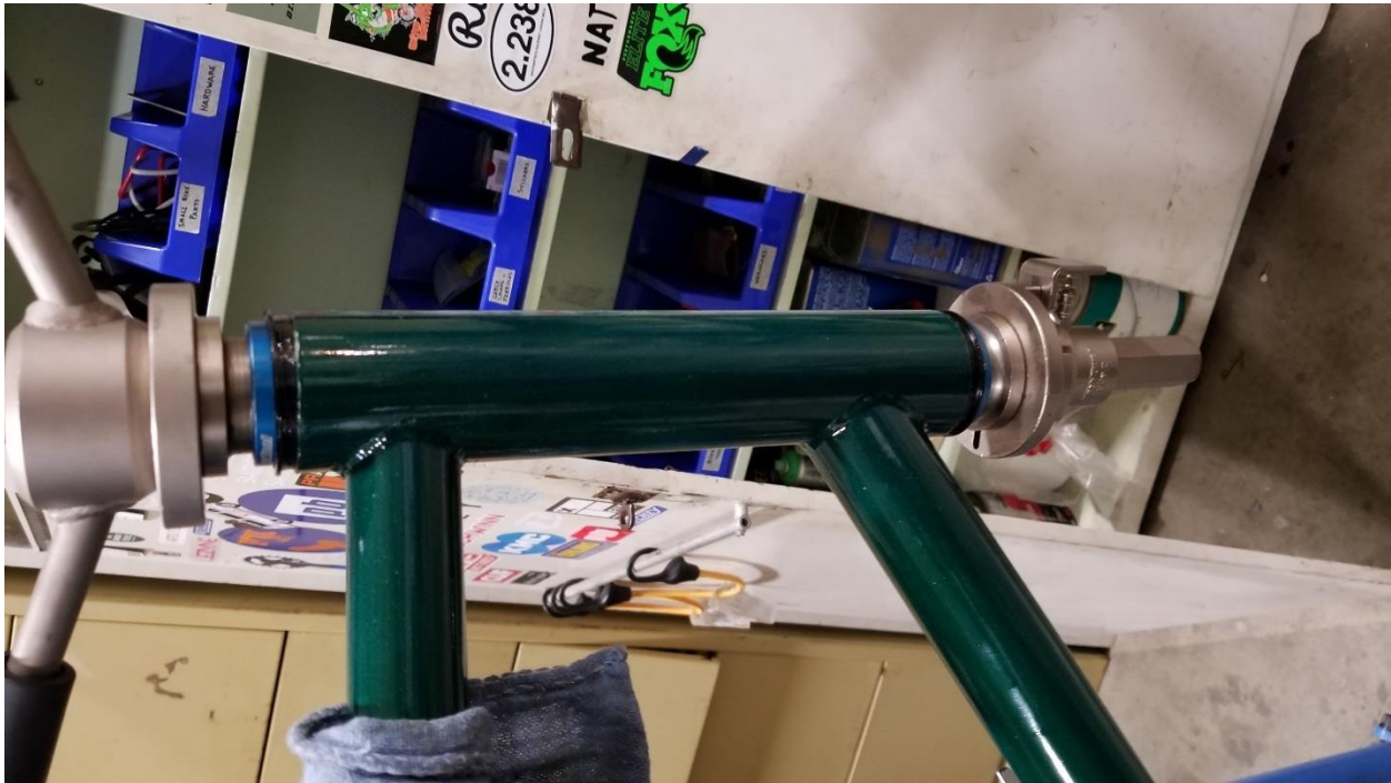
Figure 148. Facing and reaming the head tube
