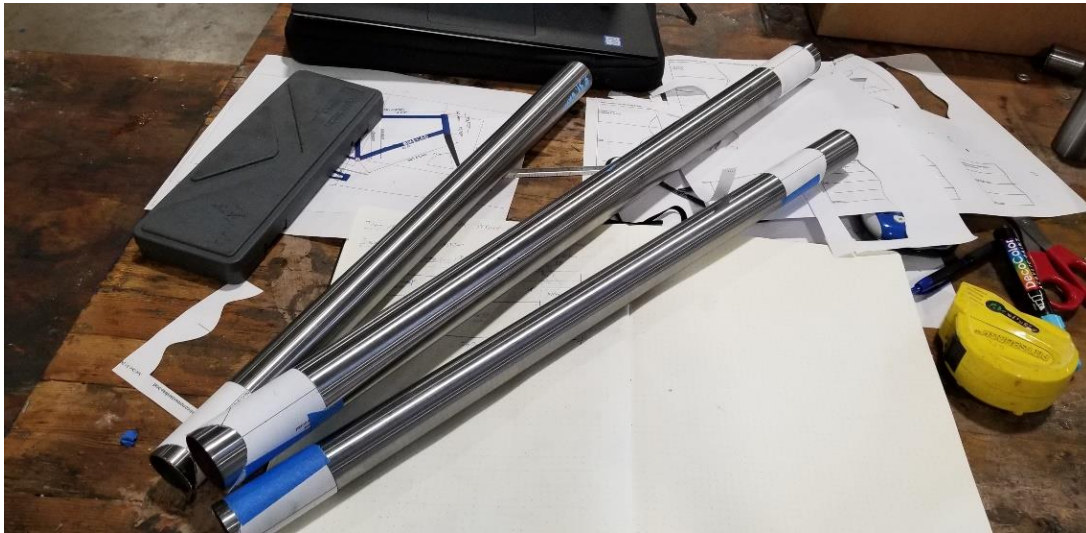
Figure 133. Unmachined tubes with miter templates taped on each end
