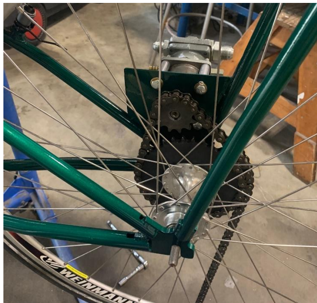
Figure 166. Rear drivetrain assembled and chain being sized 2
