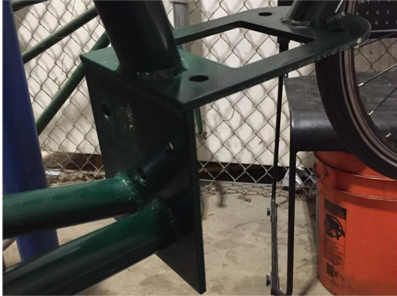
Figure 10. Bottom welded plates used for mounting the bevel gear set and planetary coupling
