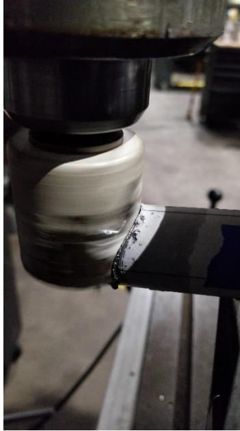
Figure 136. Close up of hole saw miter in tube
