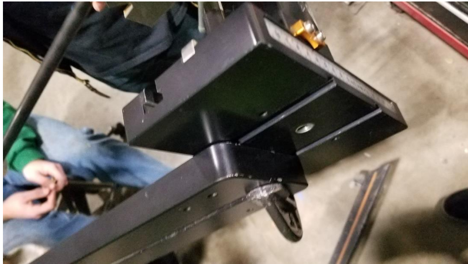
Figure 143. We had to move the rear portion of the Anvil fixture holding the rear dummy axle backwards past the normal limits of the fixture to weld the bike. We held the fixture piece to the assembly with a c-clamp.
