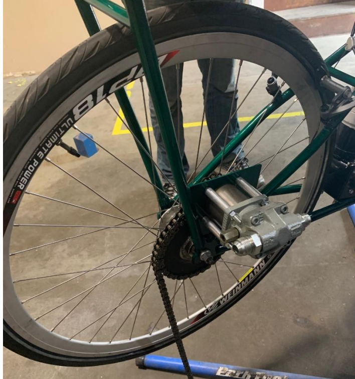
Figure 165. Rear drivetrain assembled and chain being sized
