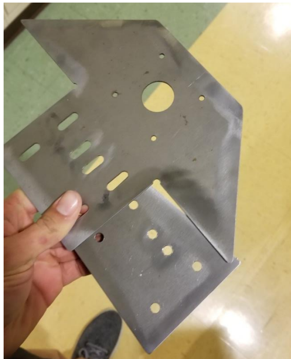
Figure 150. Front drivetrain mounting bracket flat pattern and mounting tab
