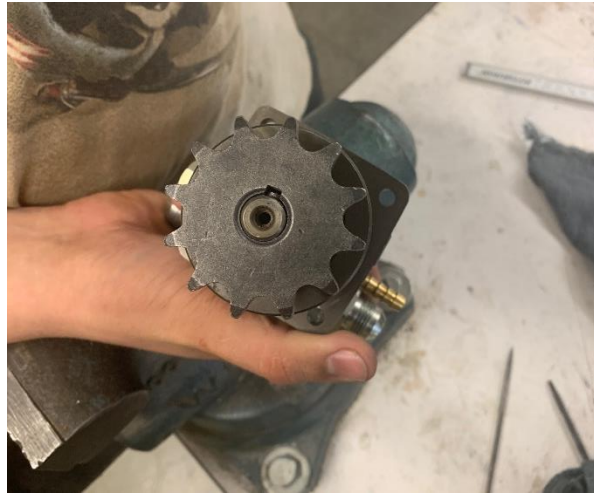
Figure 158. Broached keyway on McMaster sprocket
