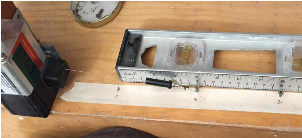
Figure 24: Calibration of Cable Extension Position Sensors
