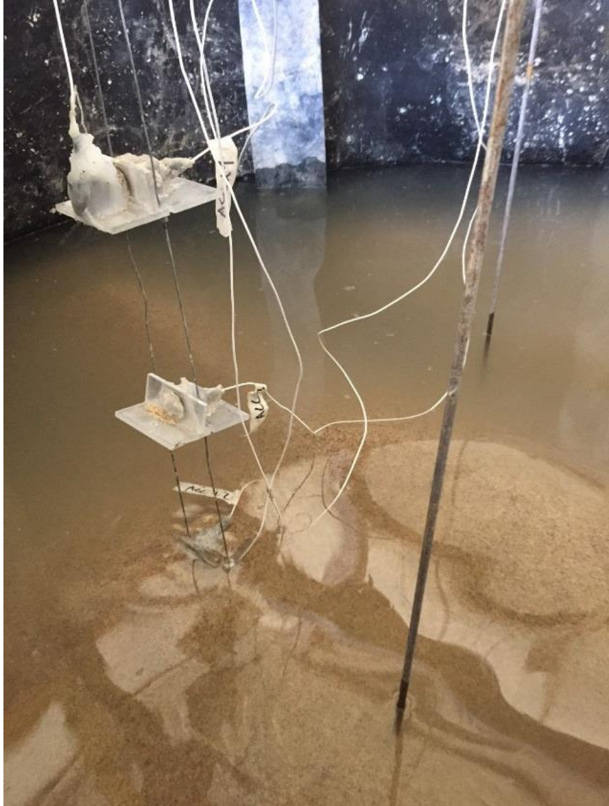
Figure 47: Accelerometer Embedment in Sand
