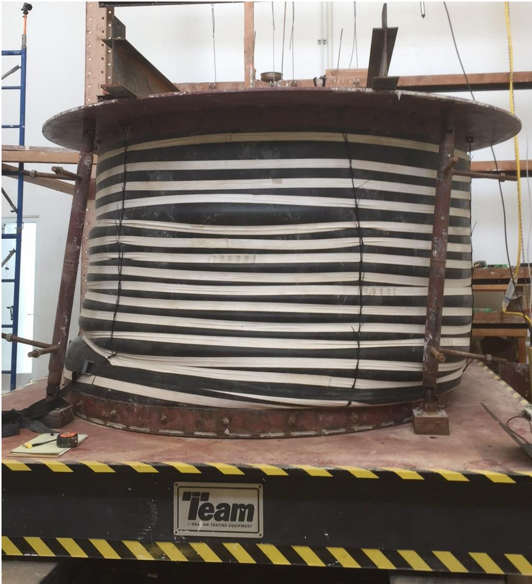
Figure 56: Displaced Bucket After Cyclic Test 1.1
