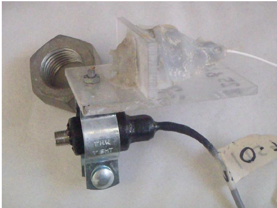
Figure 23: Pore Pressure Transducer and Accelerometer Instrument Package (From Jacobs, 2016)
