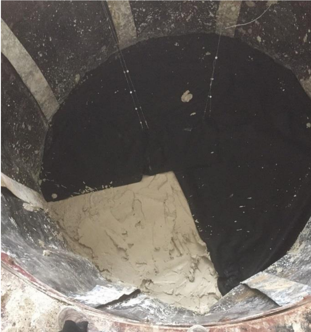
Figure 40: Clay Mixture and Filter Fabric at Base of Specimen
