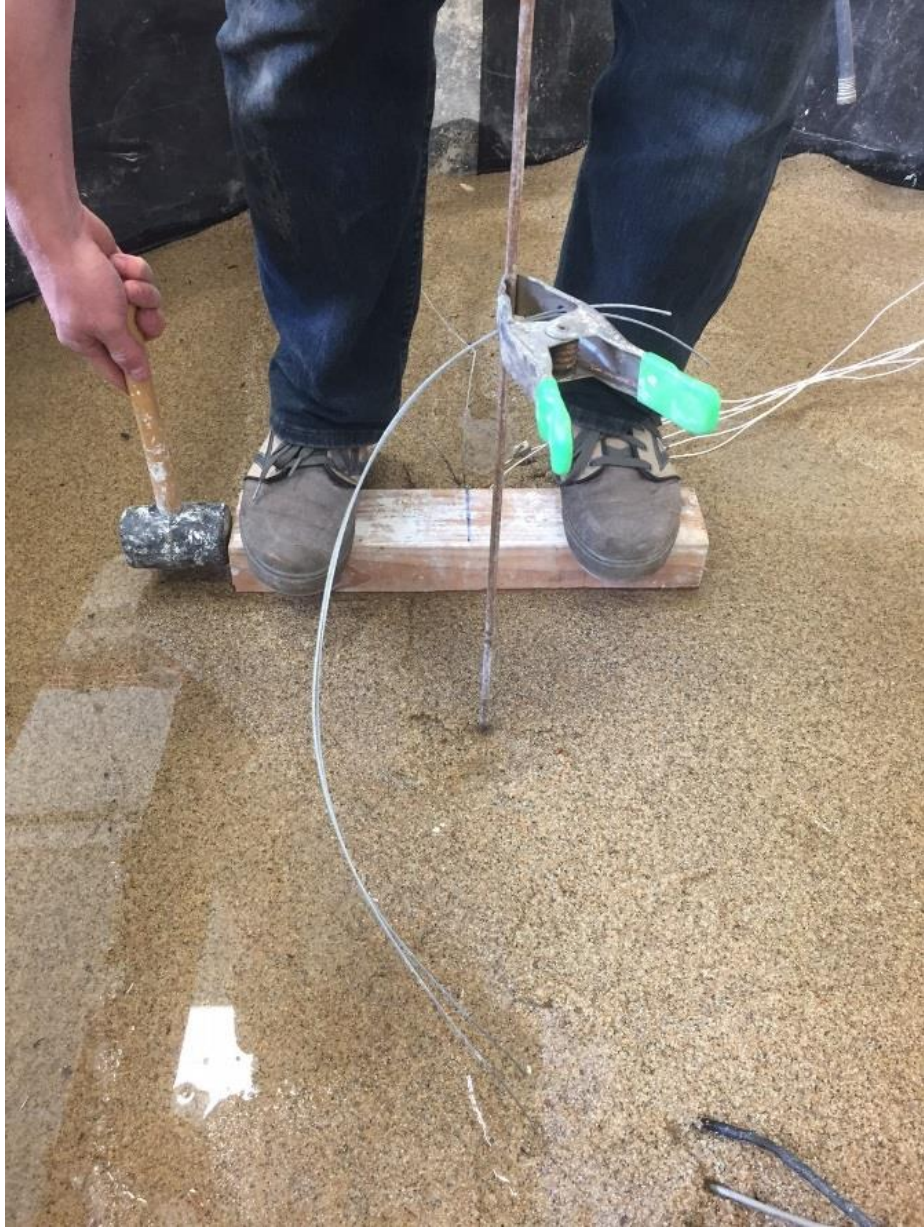
Figure 50: Shear Wave Velocity Testing
