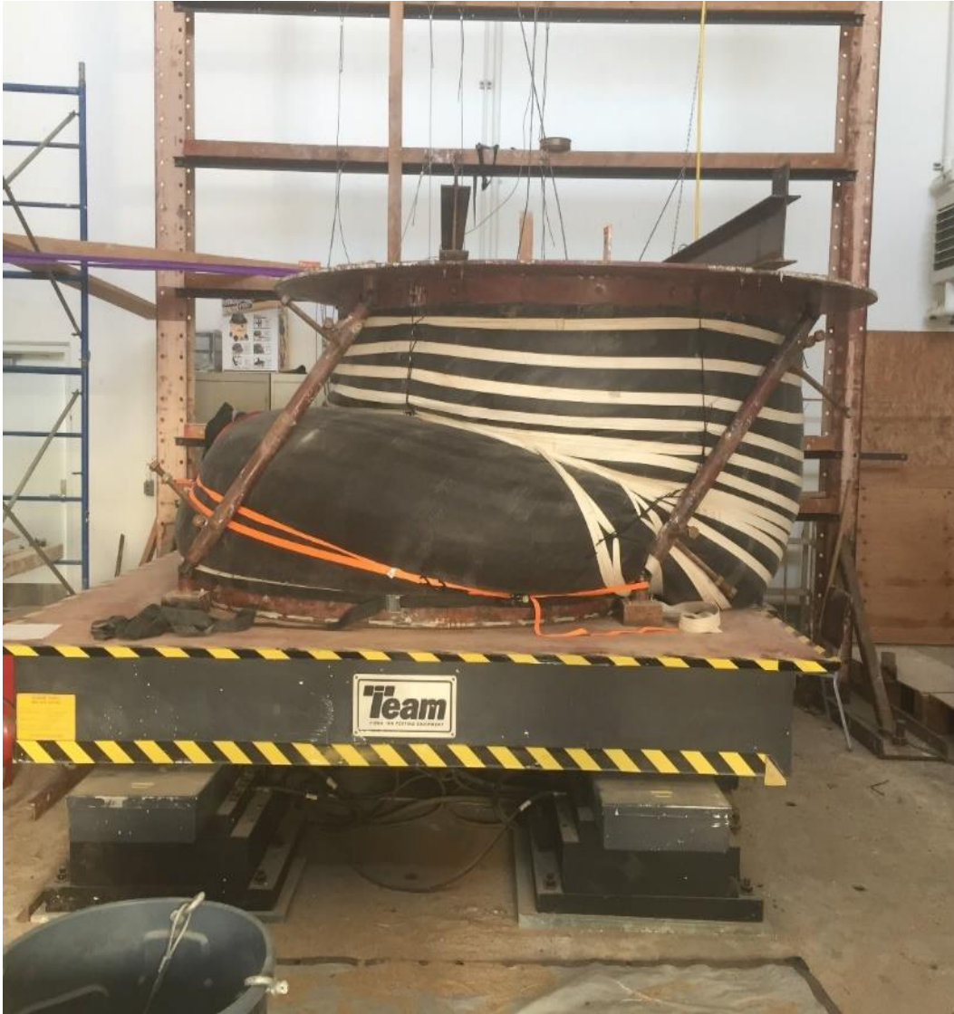
Figure 70: Displaced Bucket After Cyclic Test 2.1
