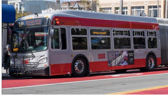
Figure 1: The new hybrid runs on B20: a blend of diesel and biodiesel which is made from recycled oil and fat. Source: SFMTA
